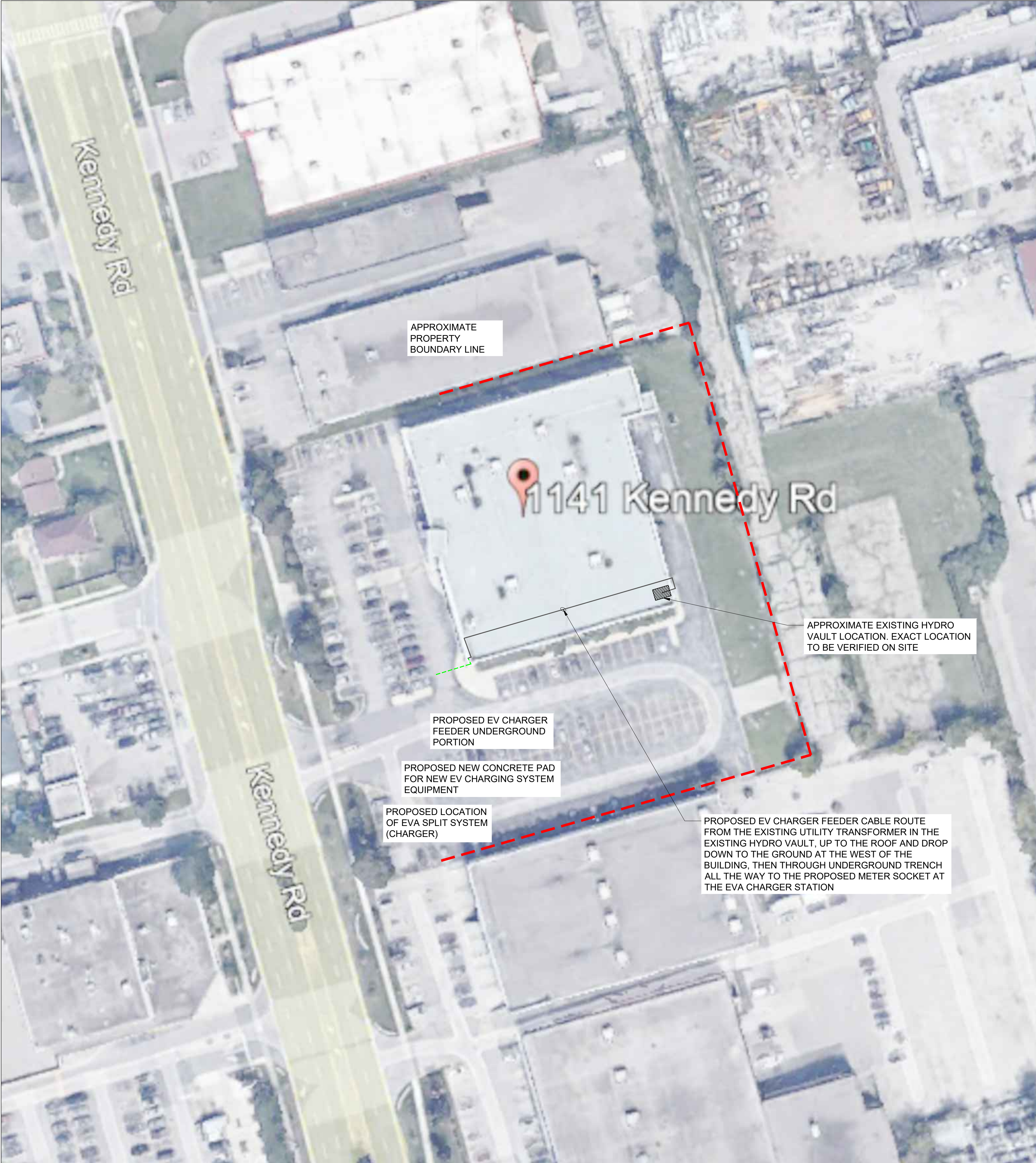
2 EV CHARGING SYSTEM INTERCONNECTION E-1 SCALE: 1:300
