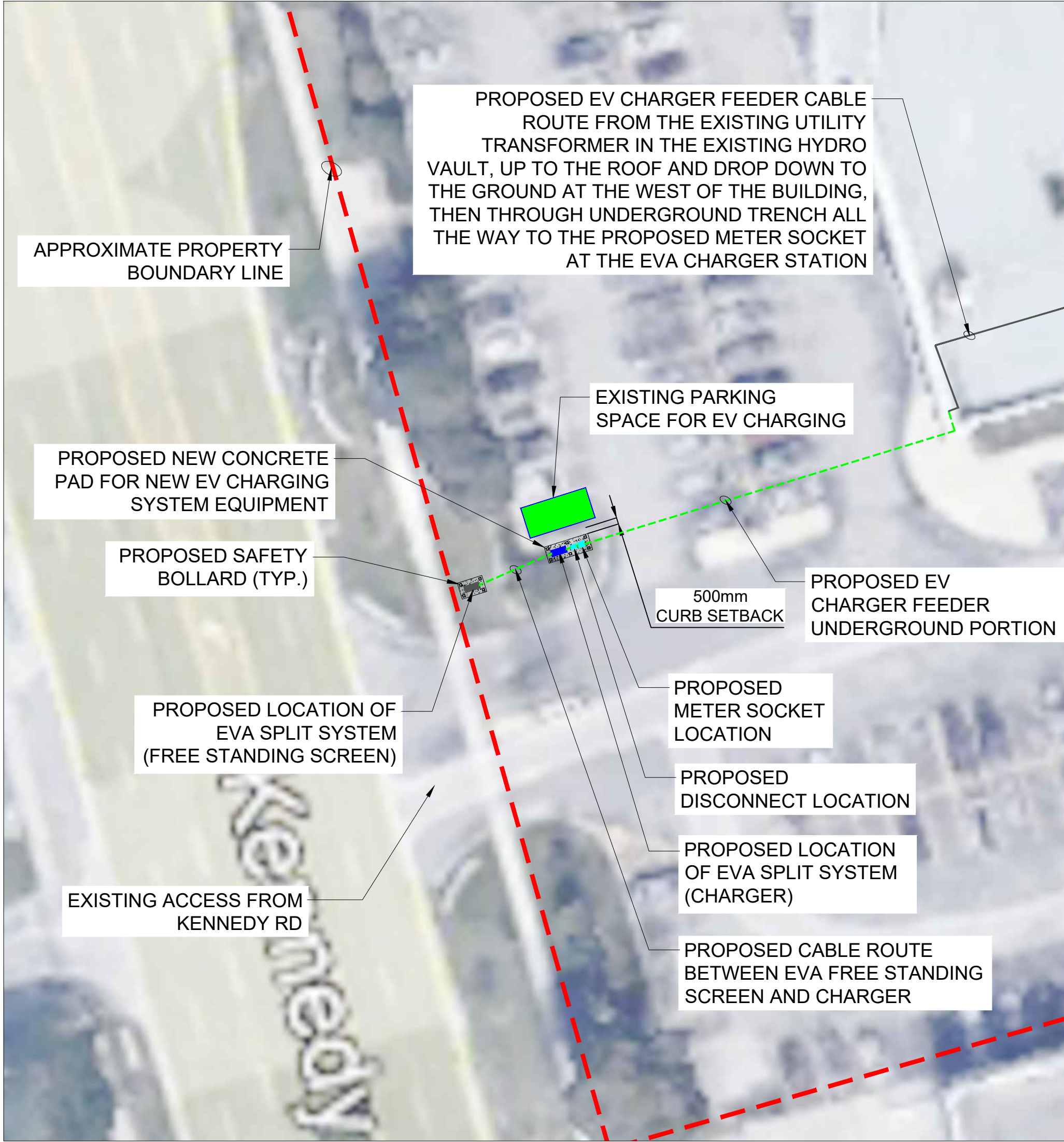
2 EV CHARGING SYSTEM INTERCONNECTION E-1 SCALE: 1:300
