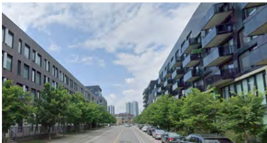
Photo of River Street near King Street East: Example of building faces that have been set back from the property line by 2-3m, with tree trunks sited at an additional 3m from the property line. This space along with soil cells have resulted in healthy tree planting.
