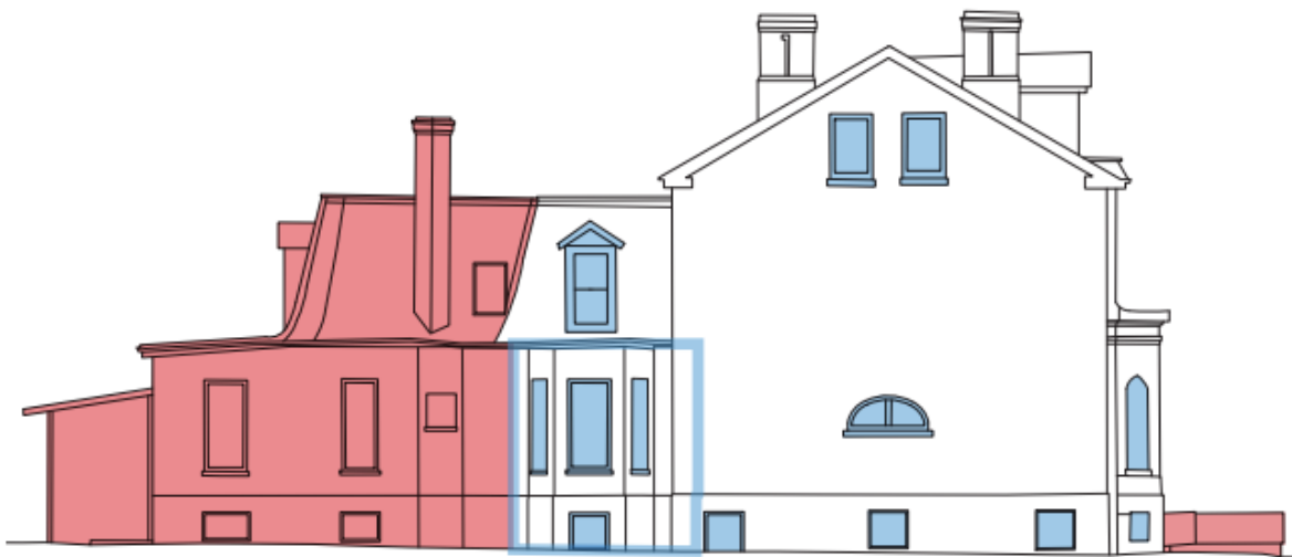
Diagram of the south elevation of 214-230 Sherbourne Street showing the portions that are proposed to be removed (ERA Architects Inc., 2024).
