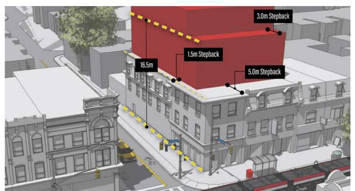
Figure 67: New development and additions to a contributing corner property shall provide a minimum stepback of 1.5 metres from the exposed side wall of the primary structure, and where their height exceeds a height of 16.5 metres, those portions of the uppermost storey shall provide an additional minimum stepback of 3.0 metres beyond the minimum 5.0 metre stepback
