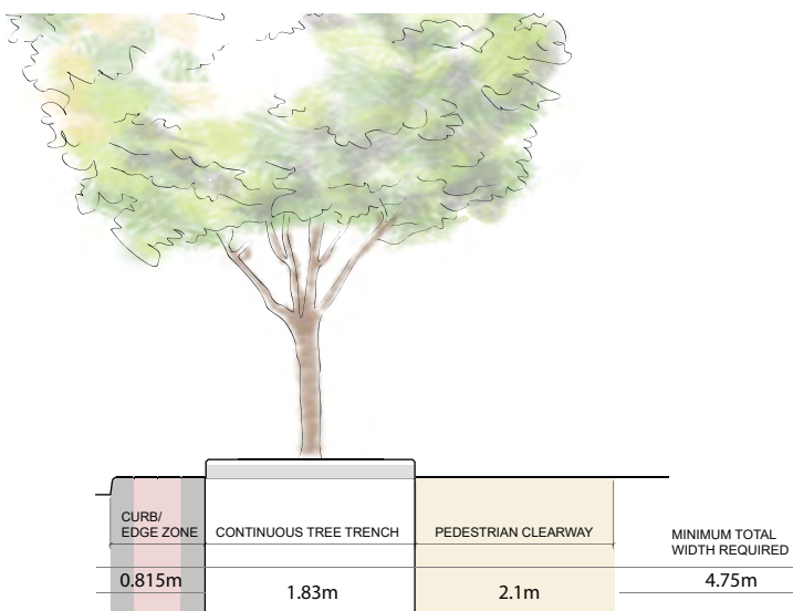
Illustration from the City of Toronto’s “Vibrant Streets: Toronto’s Coordinated Street Furniture Program” showing street tree planting details. 5
