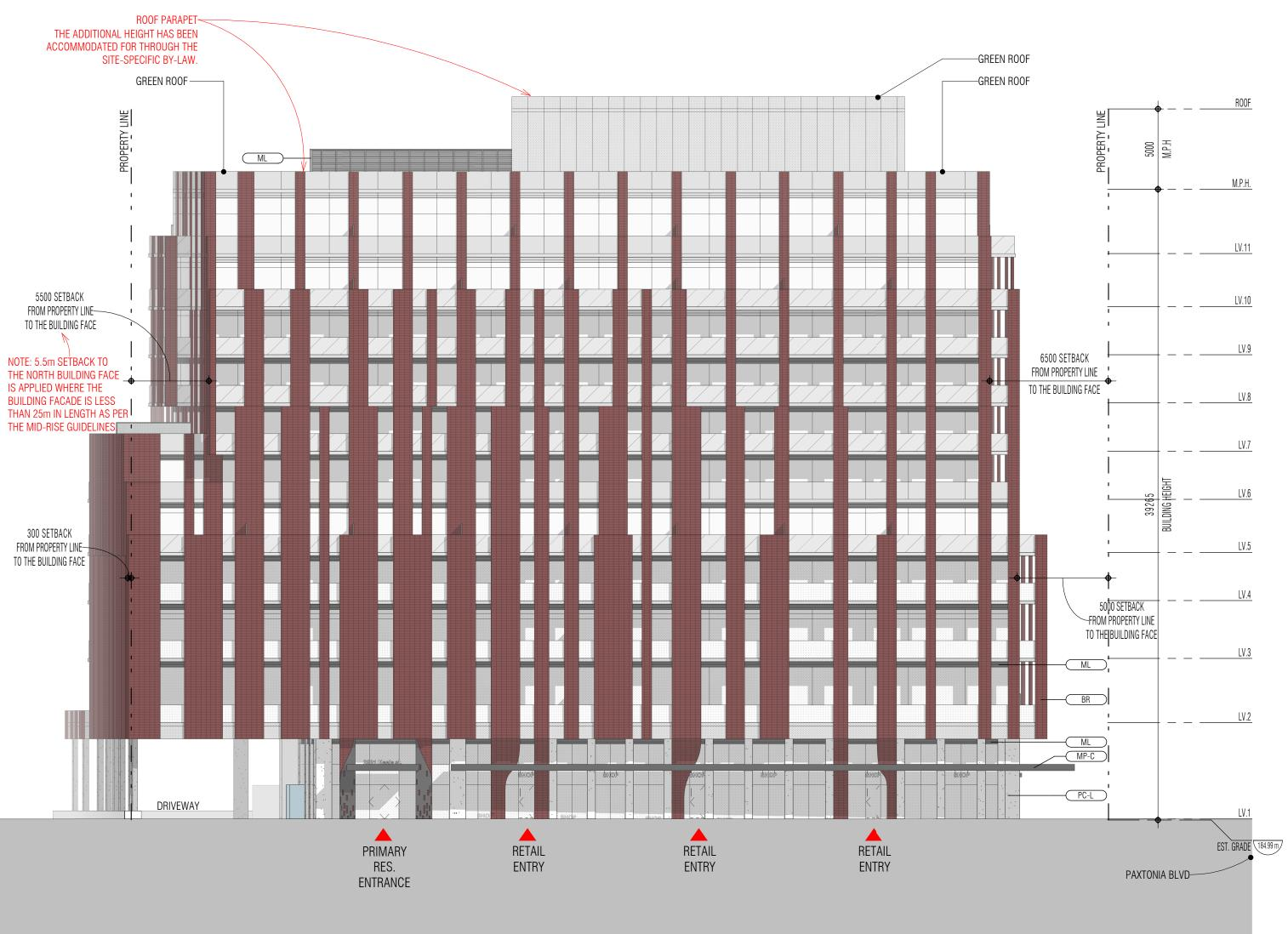
SOUTH ELEVATION 1 SCALE - 1:200 A.402
