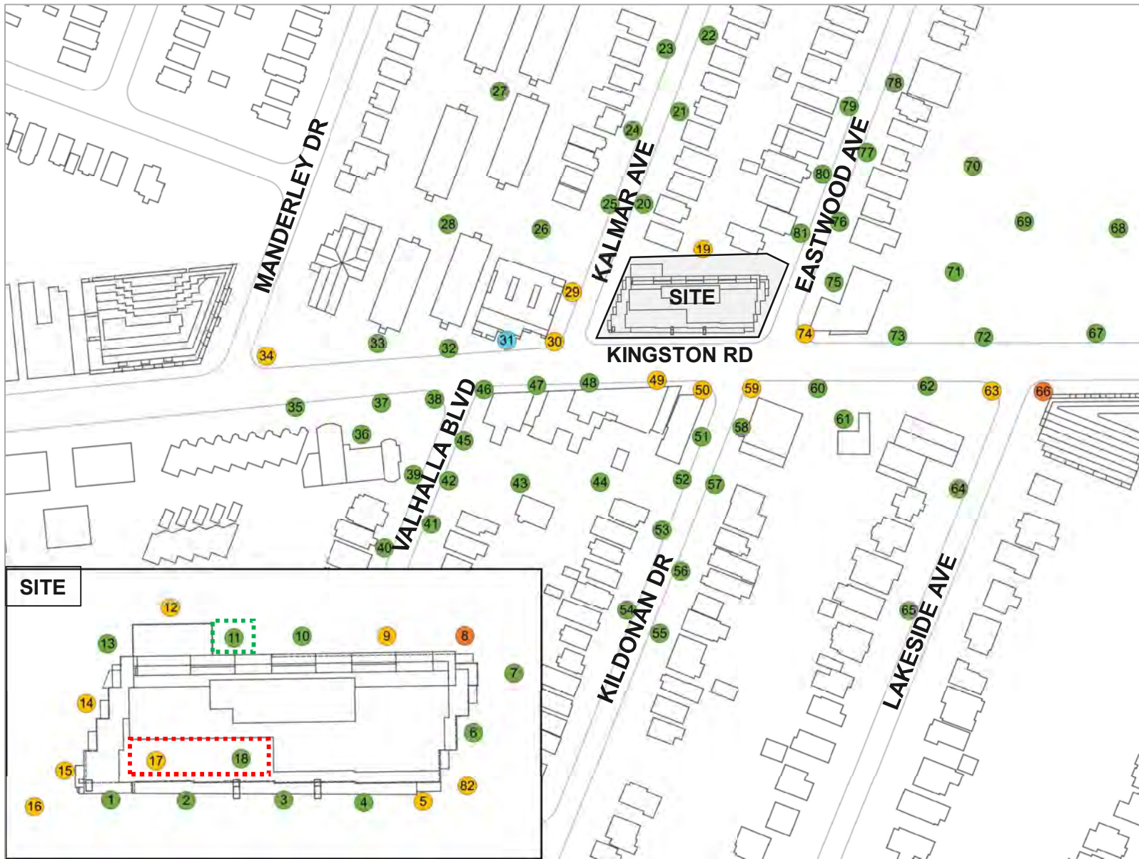
Figure 7b: Proposed Configuration – Pedestrian Wind Comfort Conditions – Winter
