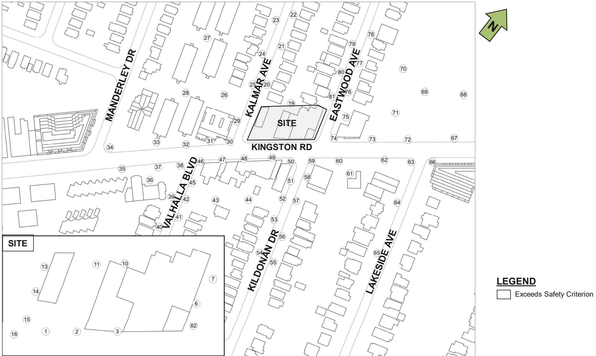
Figure 8a: Existing Configuration – Pedestrian Wind Safety Conditions – Annual
