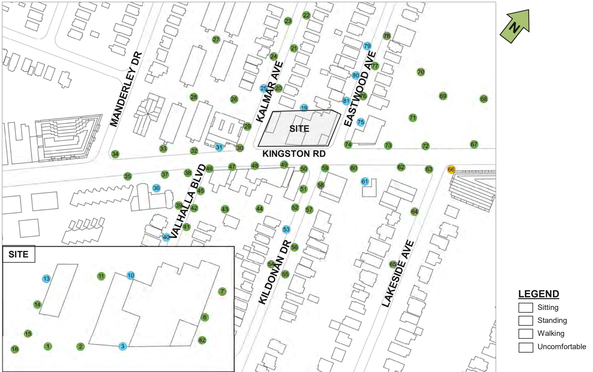
Figure A1b: Existing Configuration – Pedestrian Wind Comfort Conditions – Autumn
