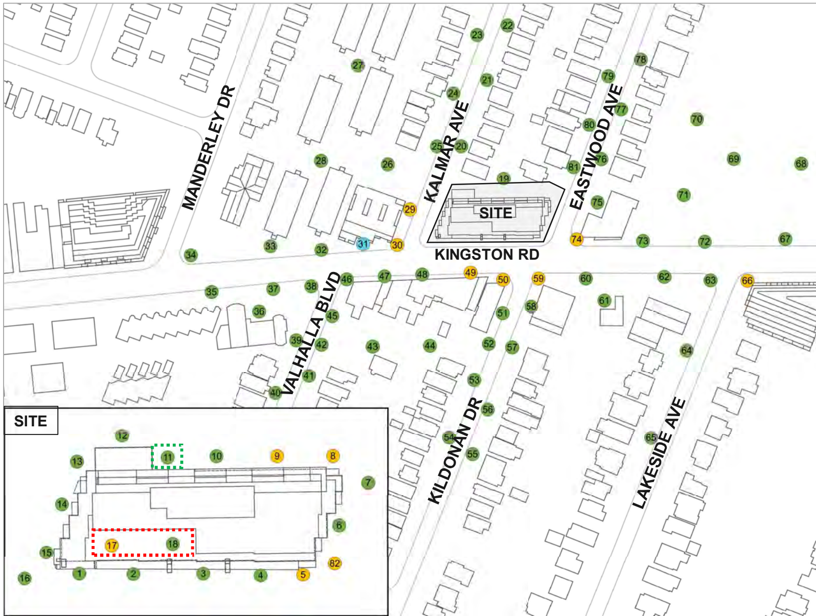
Figure A2a: Proposed Configuration – Pedestrian Wind Comfort Conditions – Spring
