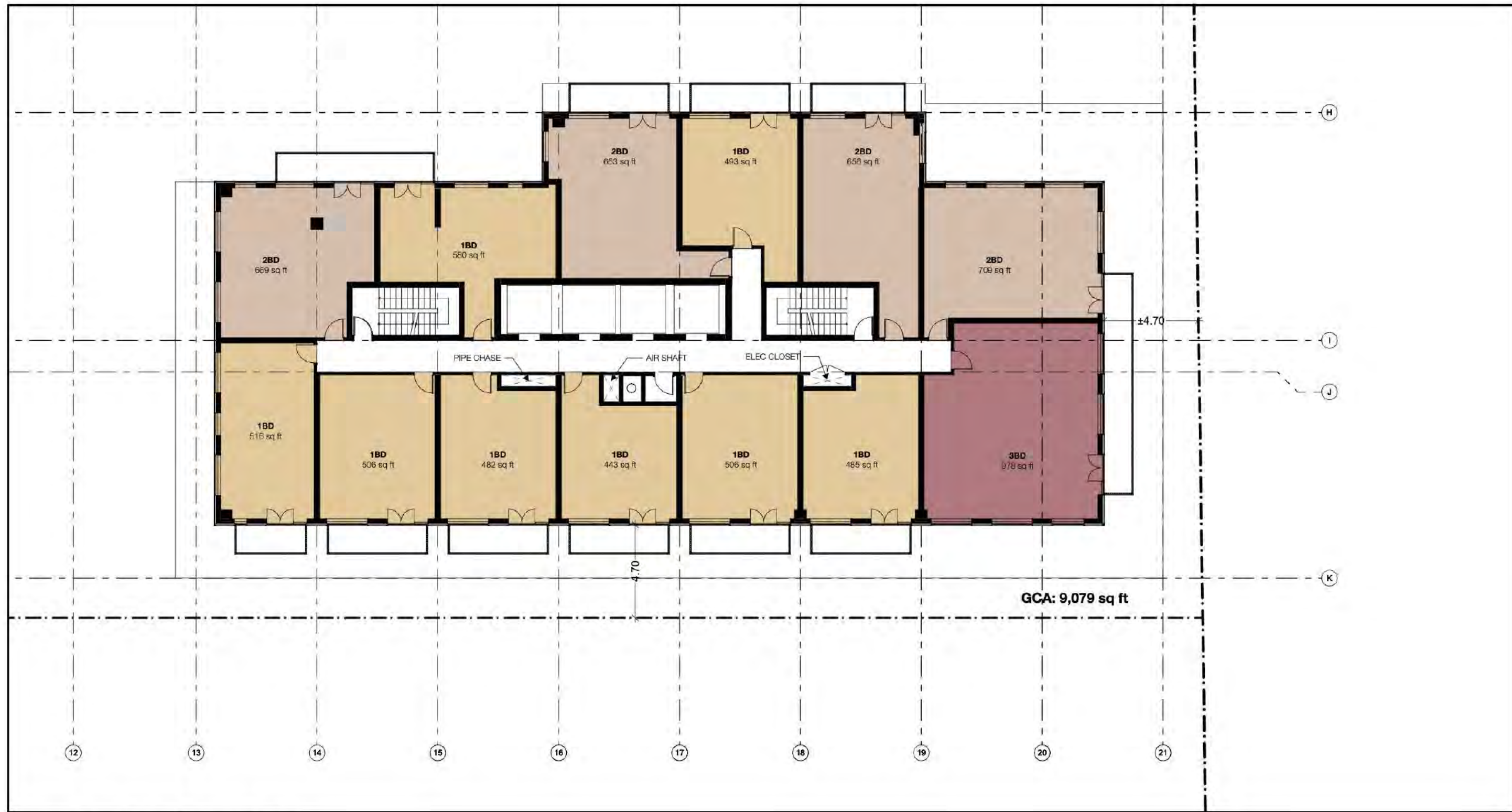
1 2D - Typical Tower Floor
