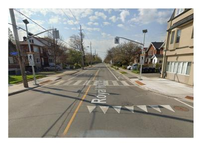
Transportation Services is also adding Level 2 PXOs to the City. **Level 2 PXOs** function the same way as a Level 1 PXO but they have different flashing lights on the side. Instead of overhead yellow Xs, there are white signs with a pedestrian symbol.
