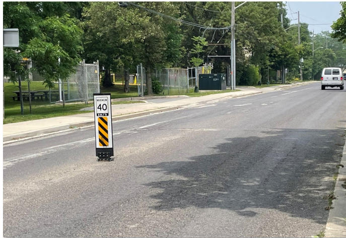
Figure 4: In-Road Flexible Speed Sign
