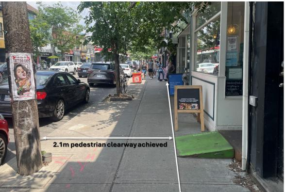
These images illustrate proper placement of a temporary ramp that meets the minimum clearway requirement, features high contrast, includes cane-detectable elements, and aligns with the landing at the top.
