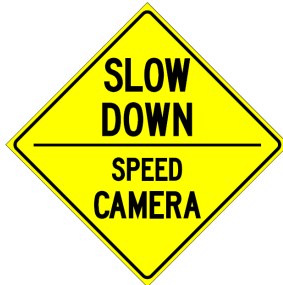
Figure 2: New ASE Warning Sign
