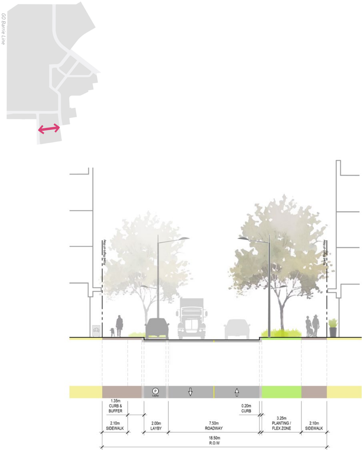
Figure 73: Conceptual cross section of Street F
