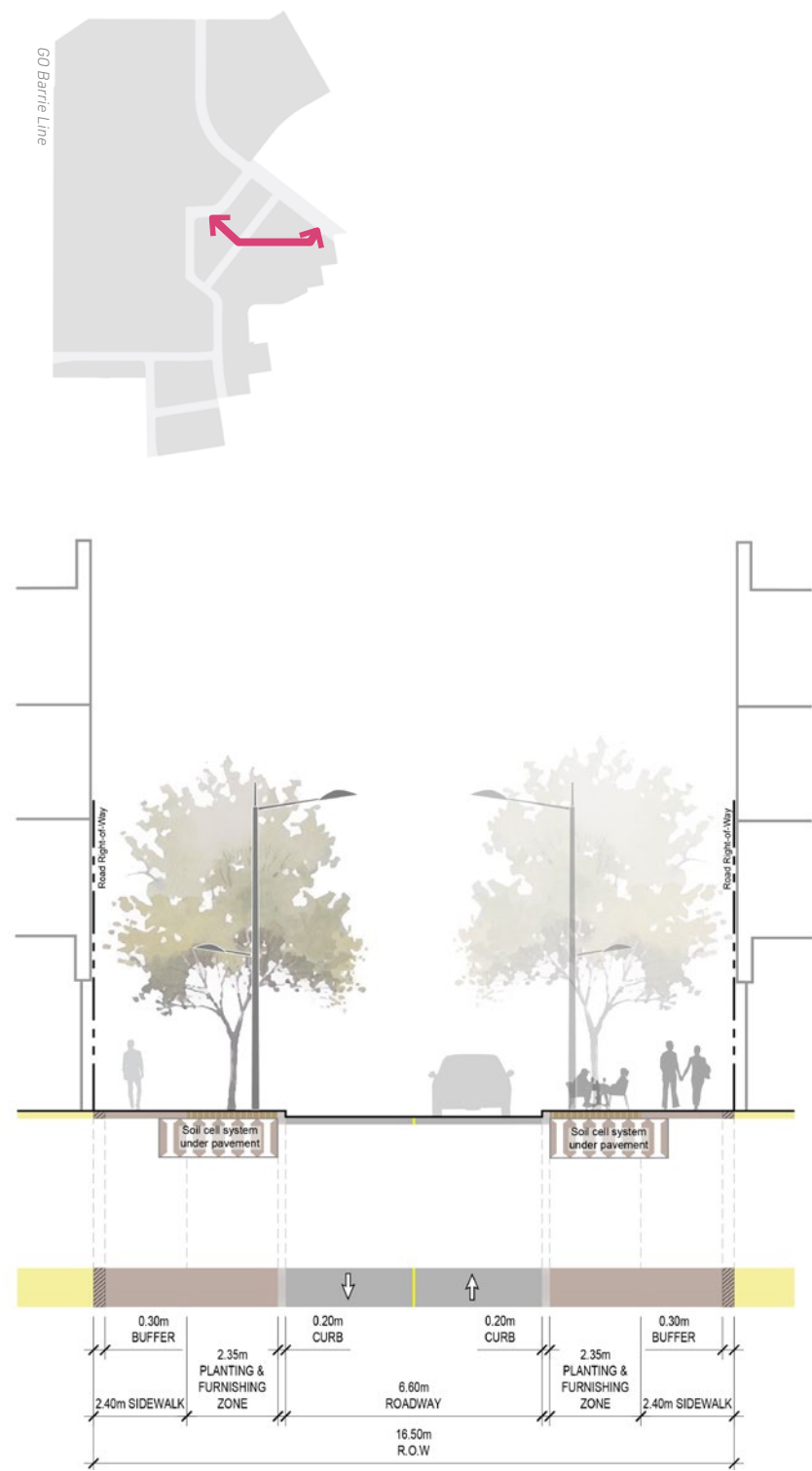
Figure 70: Conceptual cross section of Street C
