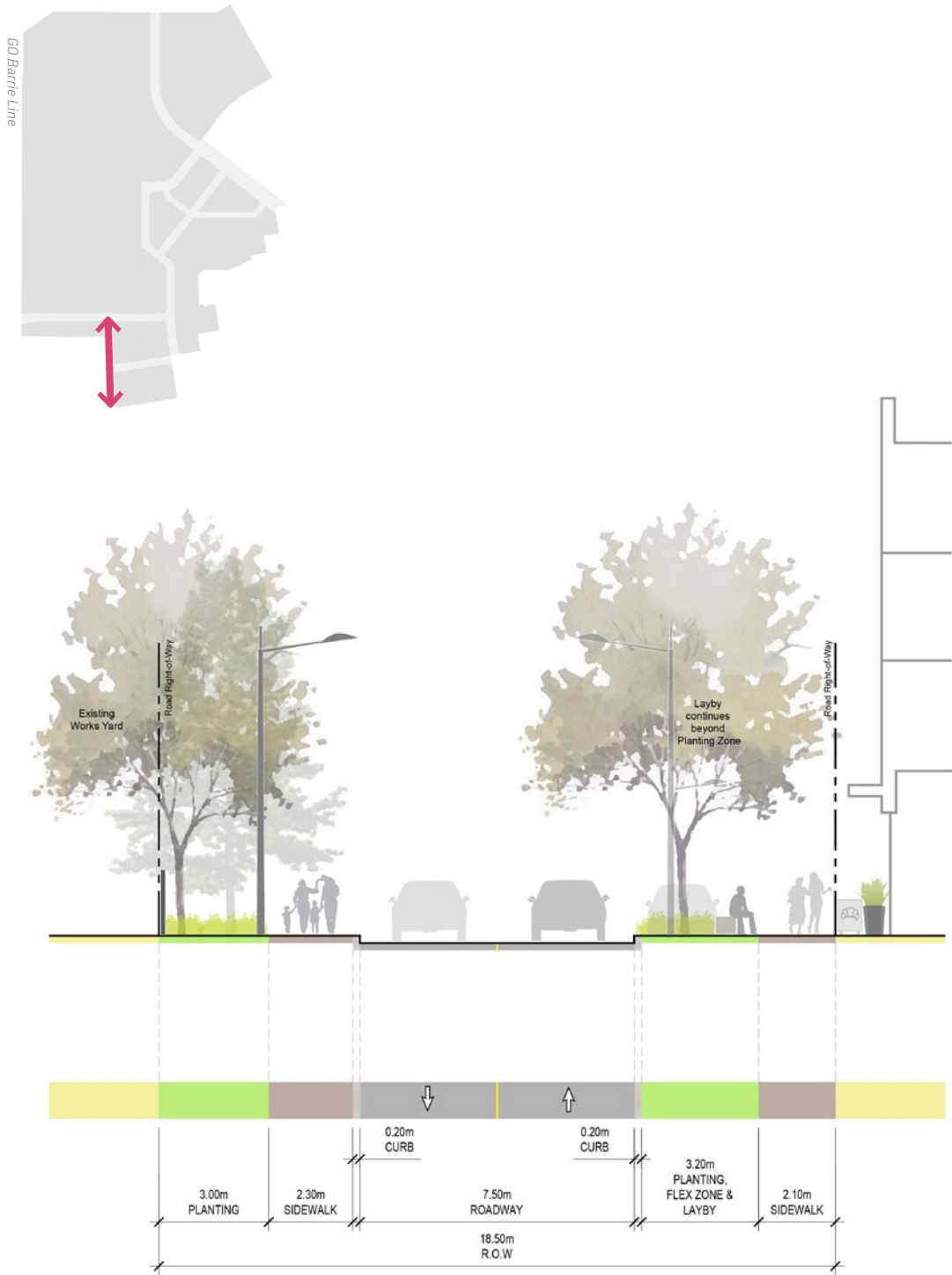
Figure 74: Conceptual cross section of Street G
