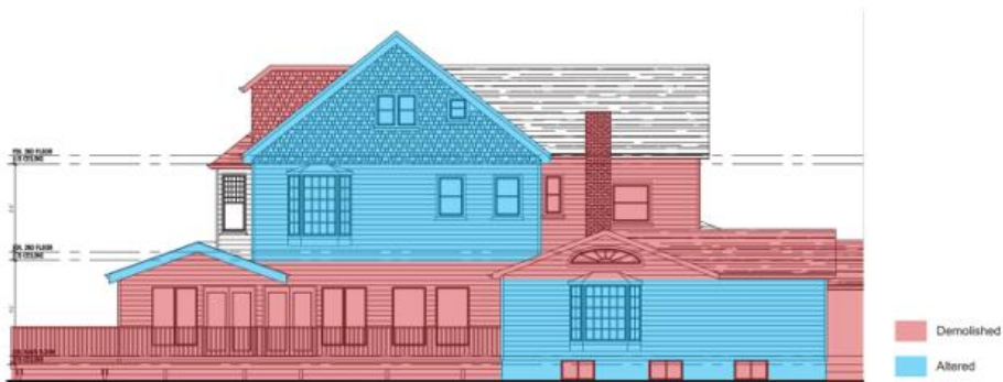
Existing and proposed west elevation of 1 Fallingbrook Road (ERA Architects Inc., Richard Wengle Architects Inc., 2024).
