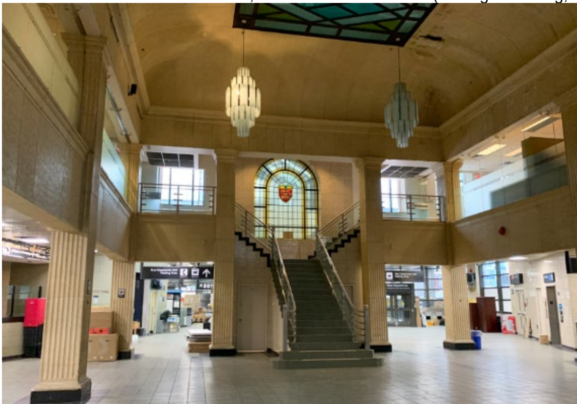
Interior of terminal building showing the centrally located, 3-bay wide, double-height entrance hall delimited by columns; coved ceiling and integrated laylight framing; bifurcated staircase leading up to the mezzanine and mezzanine level that encircles and visually overlooks the entrance hall (Heritage Planning, 2025)
