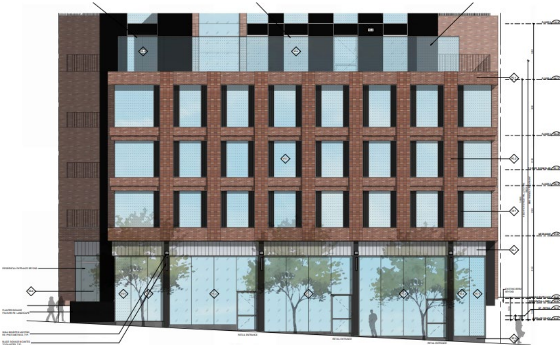
Partial south (primary) elevation showing horizontal and vertical articulation of podium building along Queen Street West and new contemporary storefront composition at the ground floor (Source: BDP Quadrangle, 2025).
