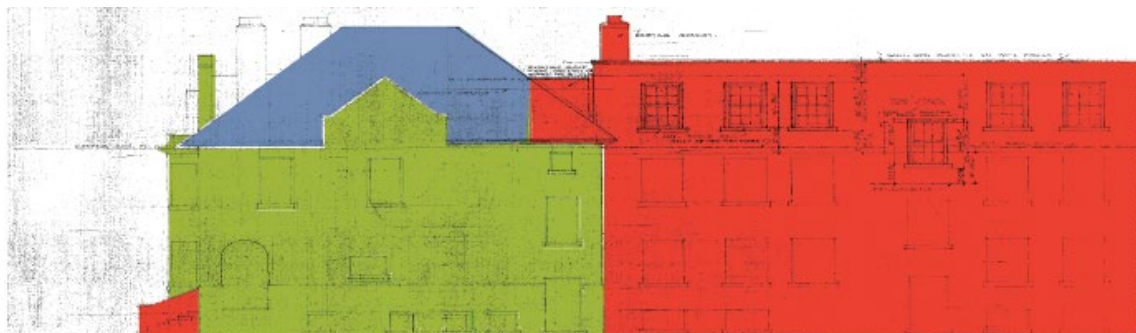
South Elevation illustrating removal of 1955 rear addition (red) with retention of the south elevation of the house (green) and reconstruction of the hipped roof (blue).
