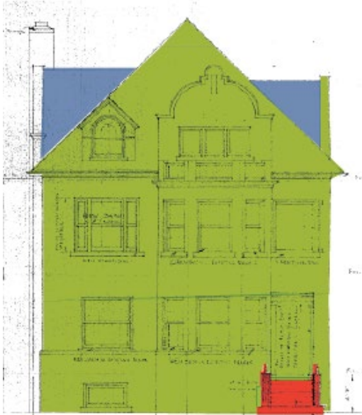
West Elevation - illustrating retention of the primary elevation (green) and reconstruction of hipped roof (blue).
