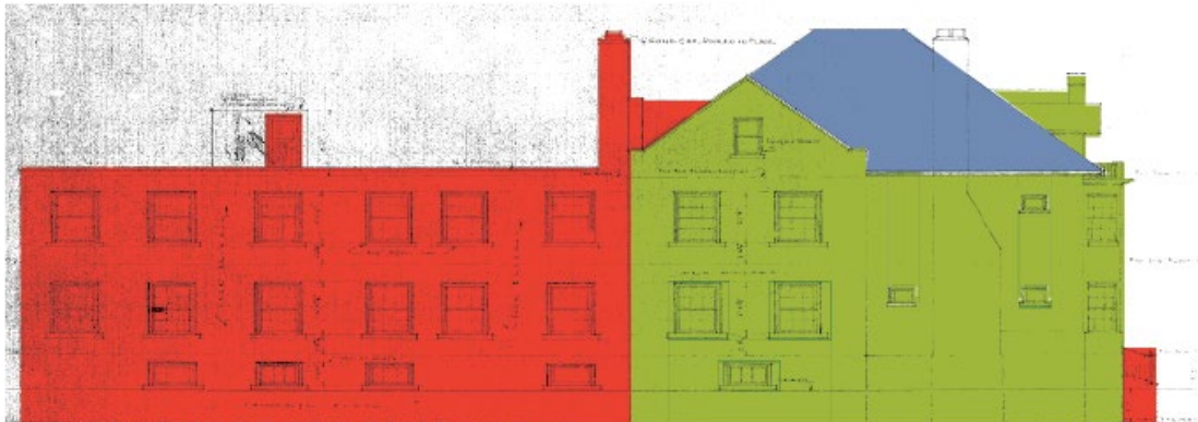
North Elevation - illustrating removal of 1955 addition to the left and retention of the north elevation of the house (green) and reconstruction of the hipped roof (blue).
