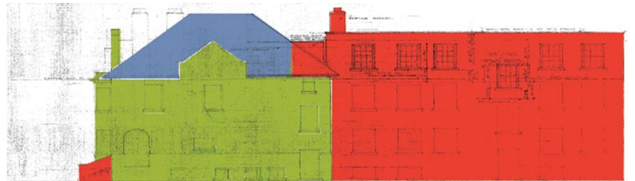
South elevation illustrating removal of 1955 rear addition (red) with retention of the south elevation of the house (green) and reconstruction of the hipped roof (blue ) 8
