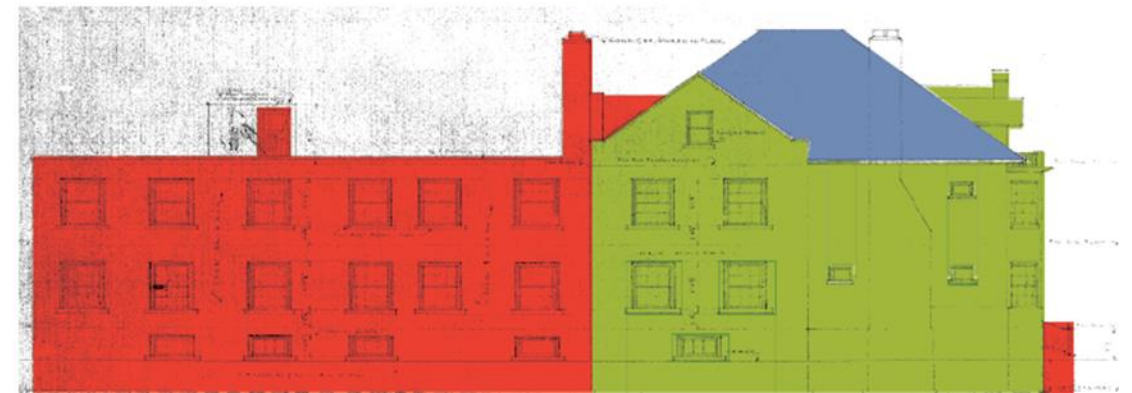
North Elevation- illustrating removal of 1955 addition (red) and retention of north elevation of house (green) and reconstruction of hipped roof (blue)
