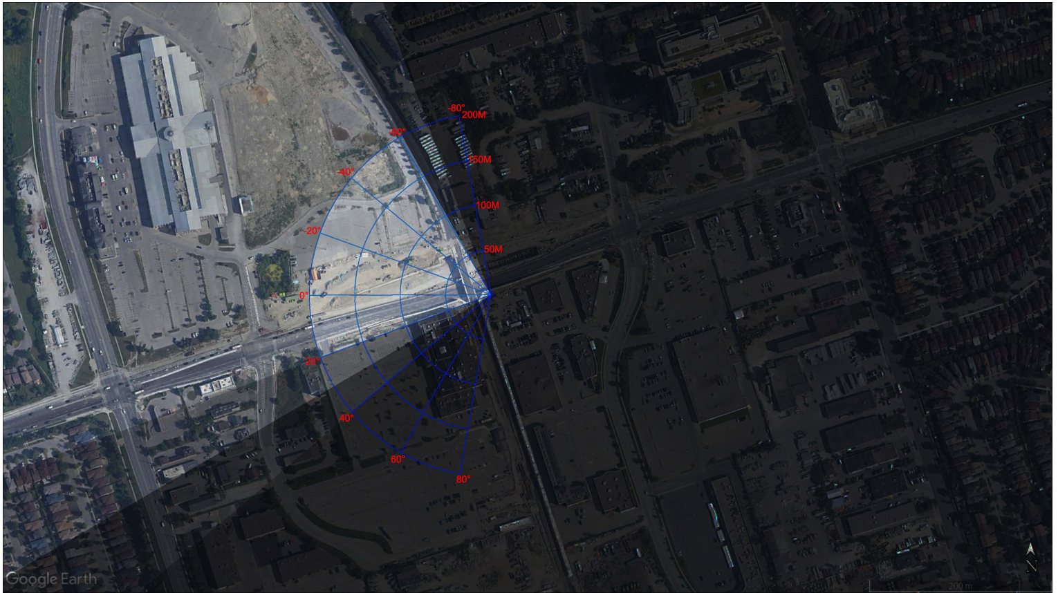
Figure 6. Site satellite photo overlay of distances and angles from proposed digital billboard site, corresponding to calculated illuminance figures in lux provided in Table 1.
