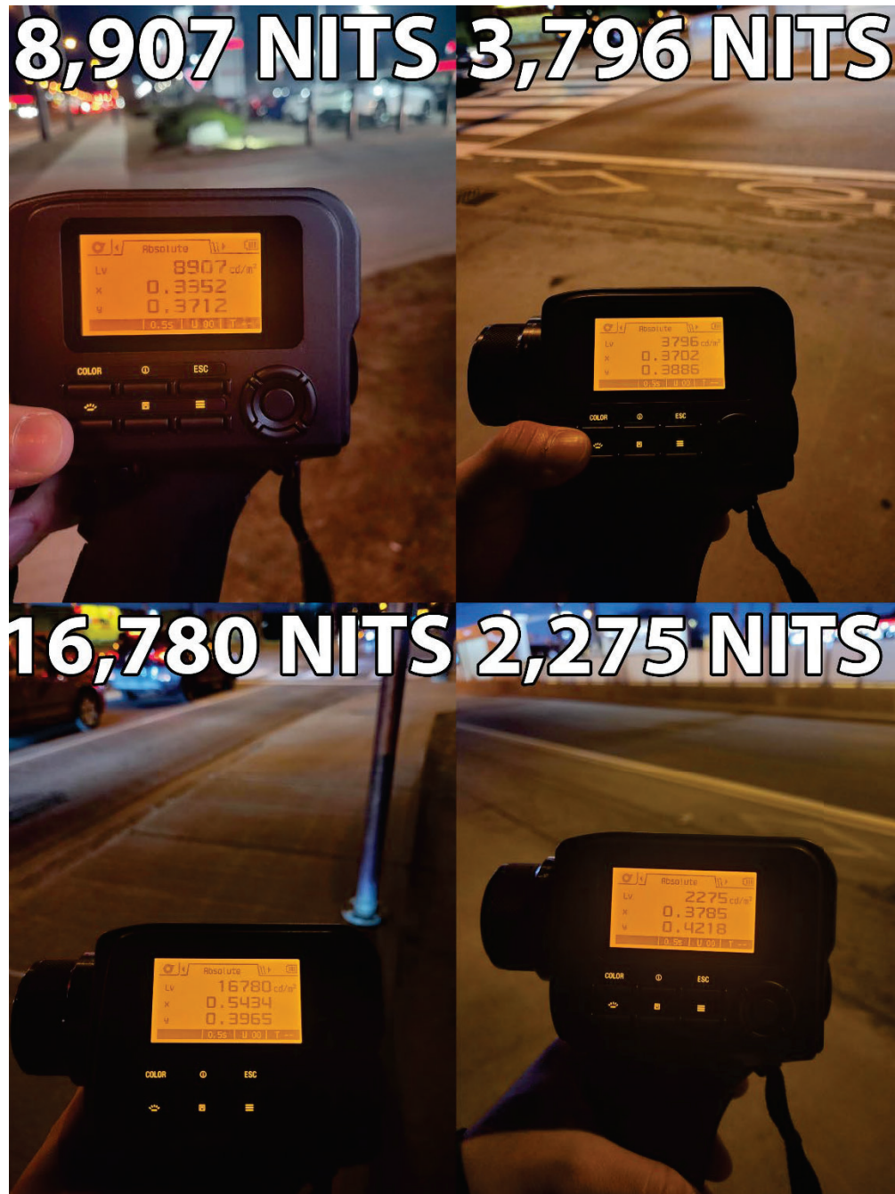
Figure 7. Field NIT measurements captured by a Konica CS-150 at various locations around the proposed area.
