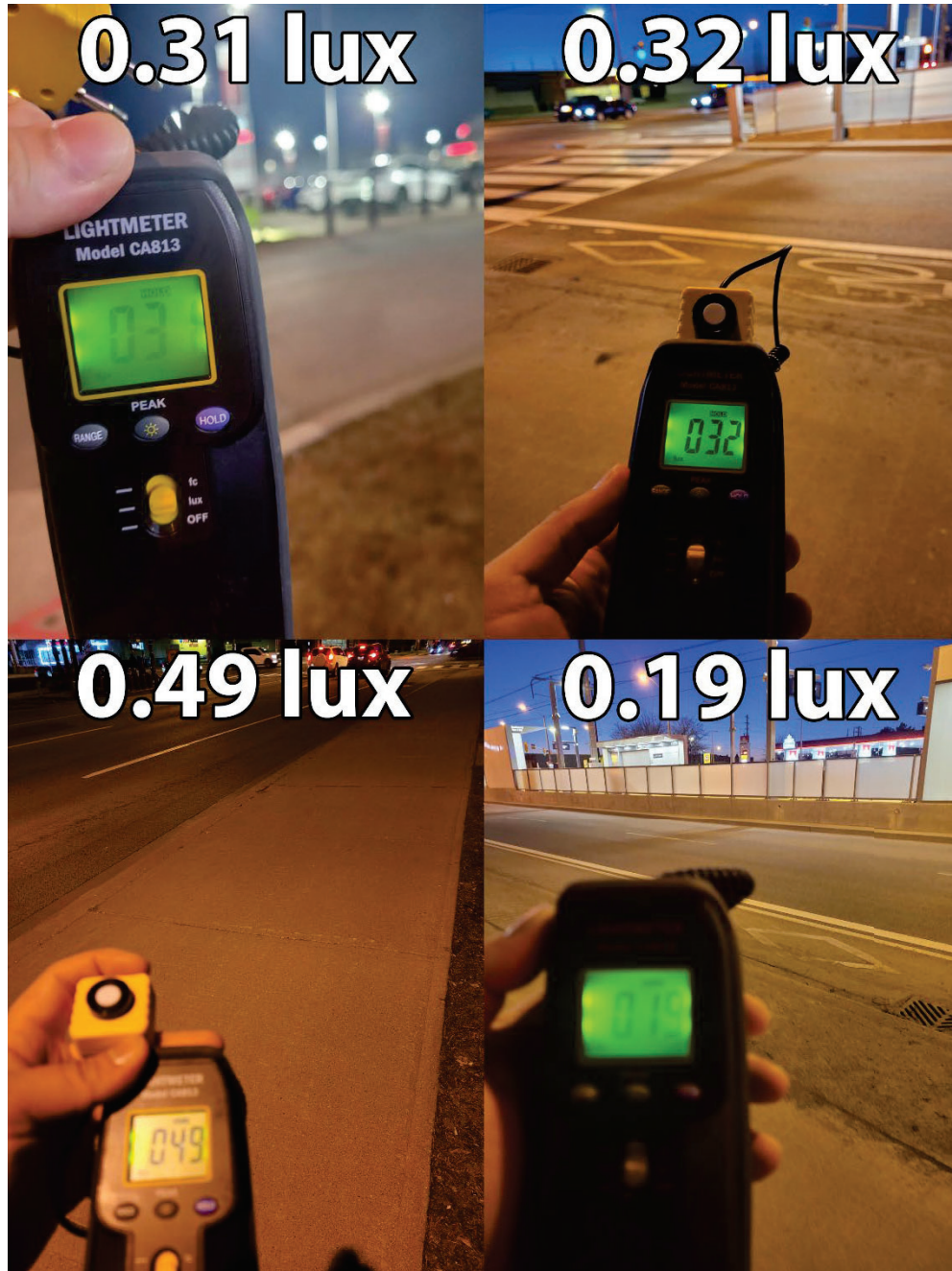
Figure 6. Field lux measurements captured by a AEMC Lightmeter CA813 at various locations around the proposed area.
