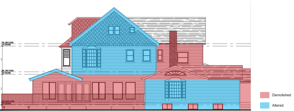
Existing and proposed east elevation of 1 Fallingbrook Road included for illustration purposes (ERA Architects Inc., Richard Wengle Architects Inc., 2024)
