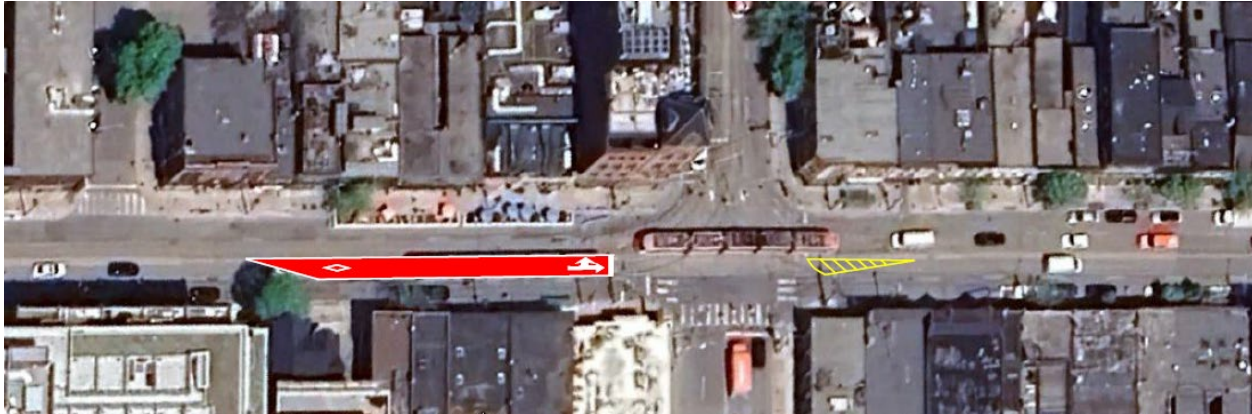
Figure 4. Schematic of reserved transit through-left lane at Queen Street East and Broadview Avenue
