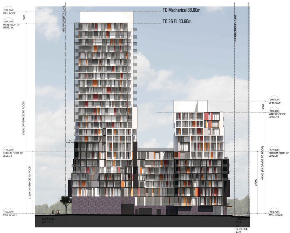
North Site West Elevation
