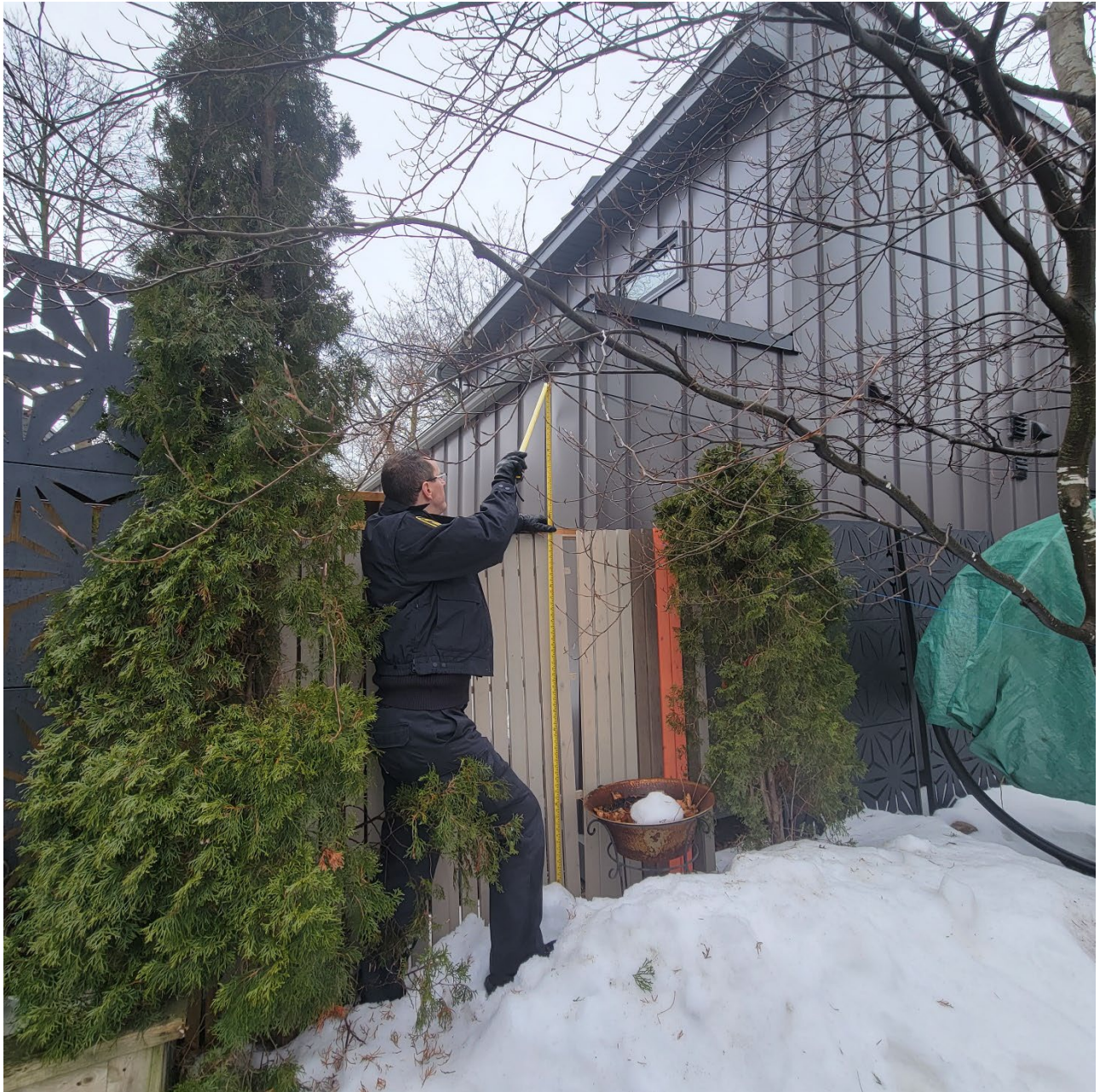
Attachment 9: Photograph depicting height measurement of 2.44 meters from grade to the top of the proposed fence. Maximum height is 2 meters .
