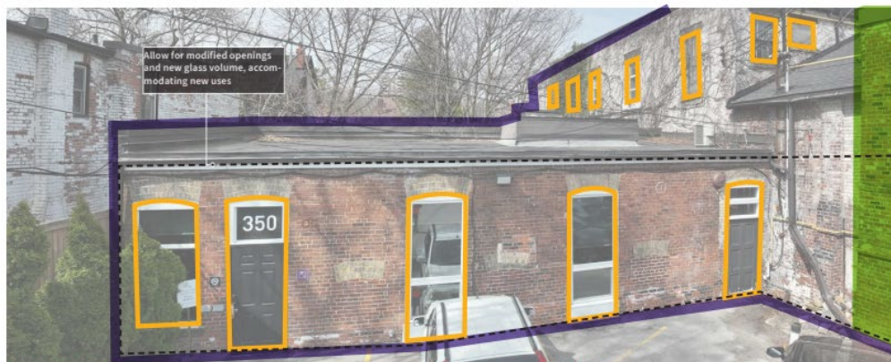
358 Dufferin Street (Core Oven Building) East Elevation Proposed Alterations and Demolitions (ERA Architects, HIA pg 81)
