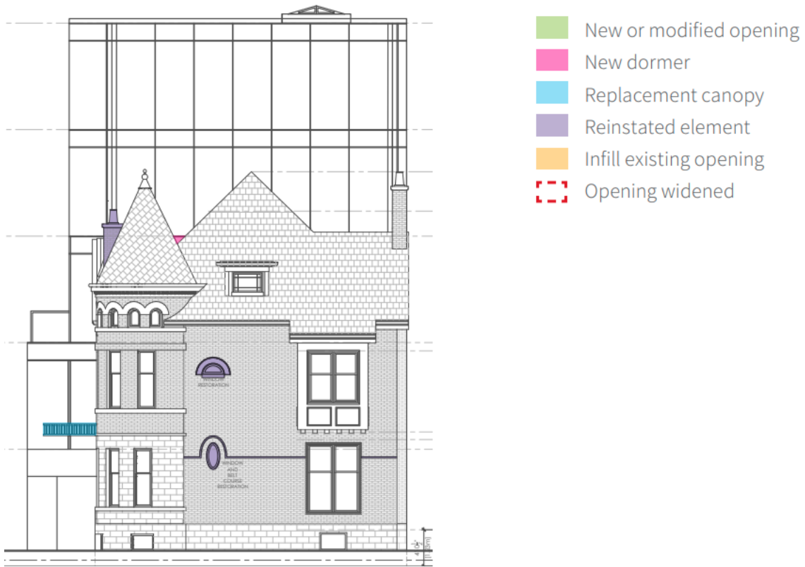
Primary (south) elevation showing the restoration of the oval window, half round window and chimney in purple and the new metal canopy on the west elevation in blue (Source: ERA Architects Inc., 2025)
