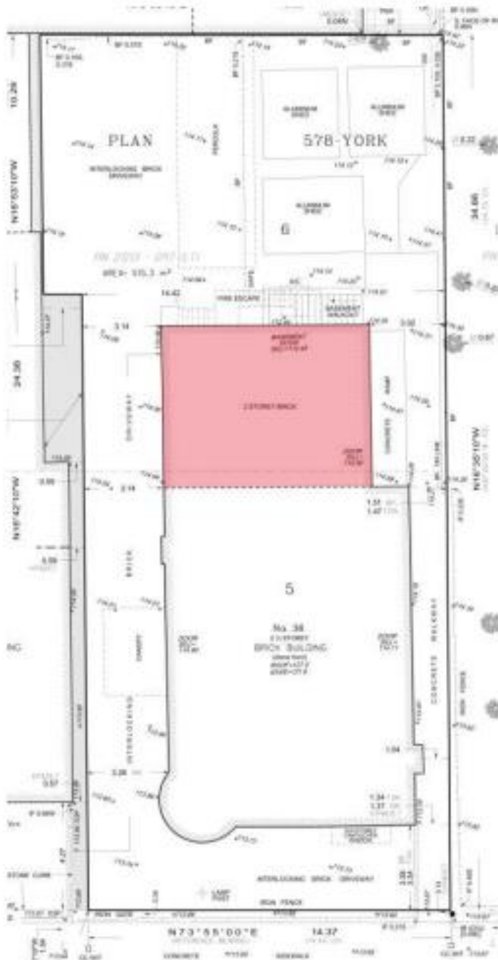
Survey of 36 Prince Arthur illustrating existing 2-1/2 storey detached brick building and 2 storey rear addition built in the 1970s in red. The later addition is proposed for demolition. (Source: ERA Architects Inc., 2025)
