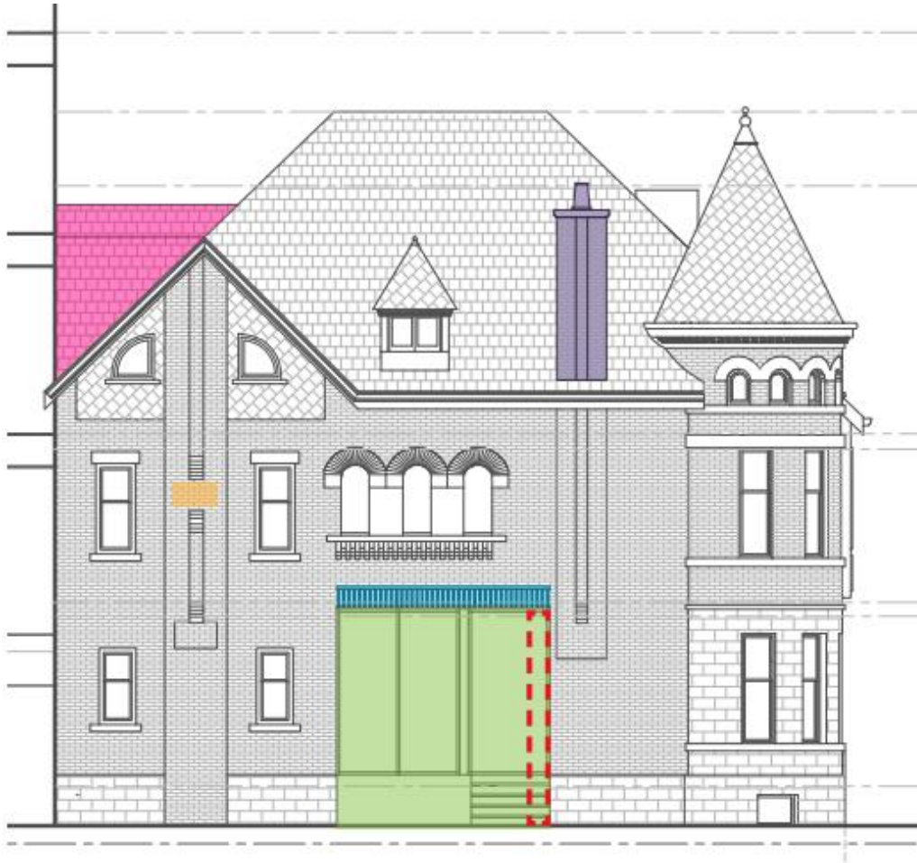
Proposed west elevation showing reinstatement of the missing chimney in purple, replacement with metal canopy in blue, new rear dormer in pink, widened entrance in green with red hash line showing area of masonry removal, and infill of vent opening in orange (Source: ERA Architects Inc., 2025)
