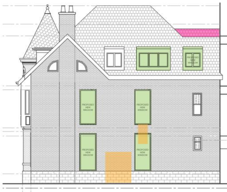
Proposed east elevation showing new windows in green, new rear dormer in pink and infilled openings in orange (Source: ERA Architects Inc, 2025)
