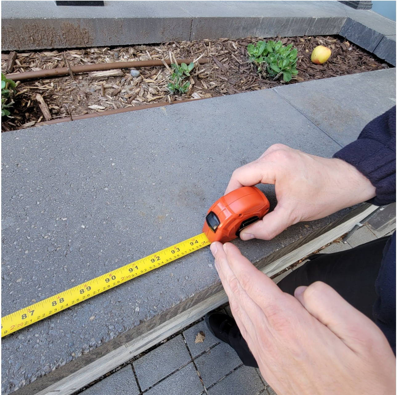
Attachment 6: Photograph depicting measurement of 2.4 meters from front lot line. Maximum height is 1.2 meters within this measurement.
