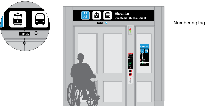
Elevator – Numbering tag Elevation 1:50
