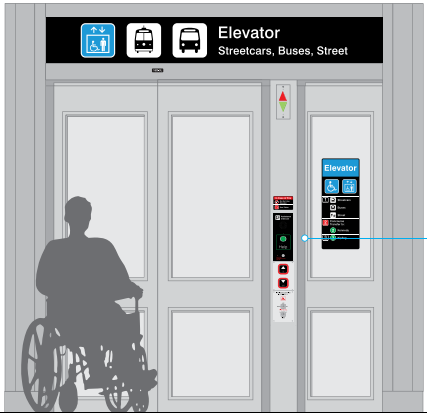
Assistance Intercom – Exterior
