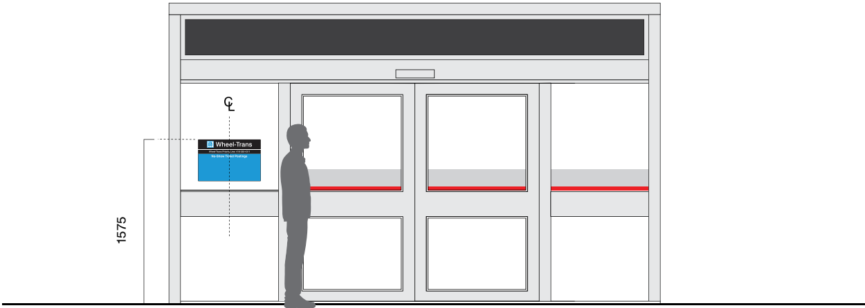
Wheel-Trans Stop – No Show Board – Interior Elevation 1:50
