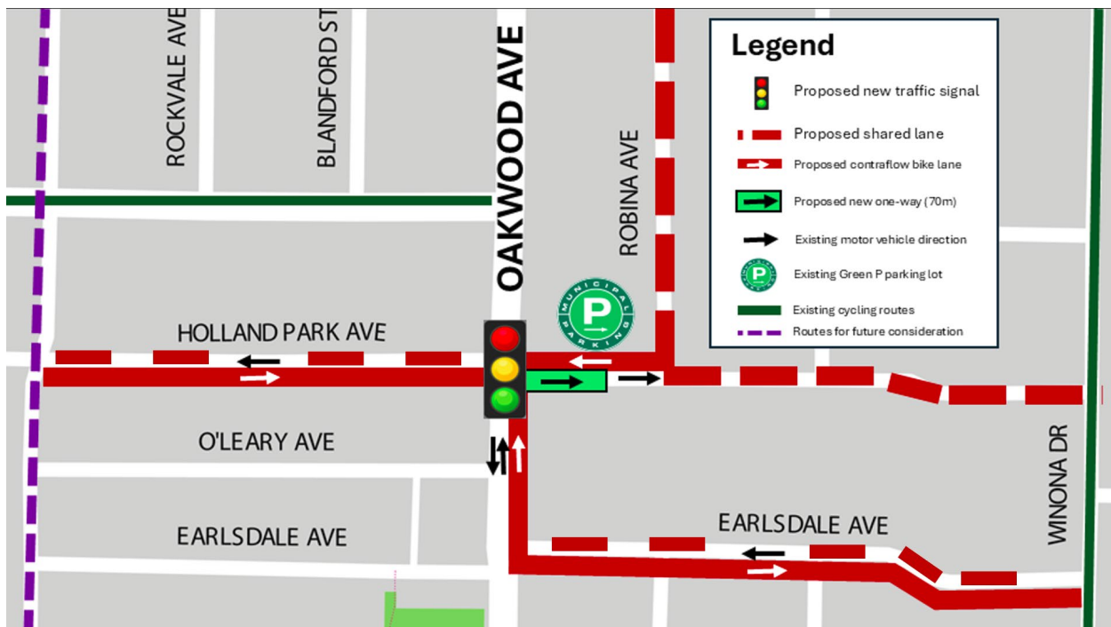
Figure 5: Map of Recommended New Traffic Signal at Oakwood Avenue and Holland Park Avenue and Proposed Changes to Cycling Routes
