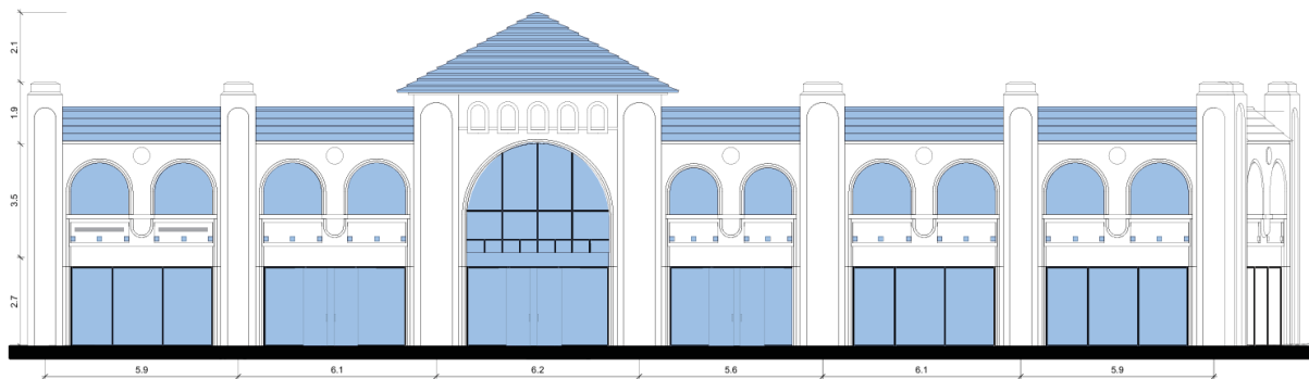
Proposed alterations in blue for the heritage façade on the west elevation (Adamson Architects, 2026, annotated by ERA Architects).
