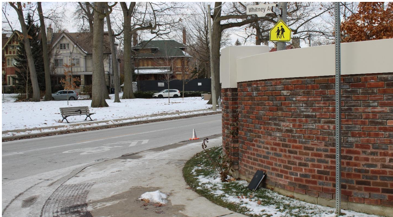
Figure 3: Site exam photo, looking north from a stopped position on Whitney Ave., with the camera 2.0 m back of the stop line, corresponding to the front bumper being stopped at the stop line. The incident brick wall limits the view of southbound vehicles to only 27 m north of the centre of this lane.
