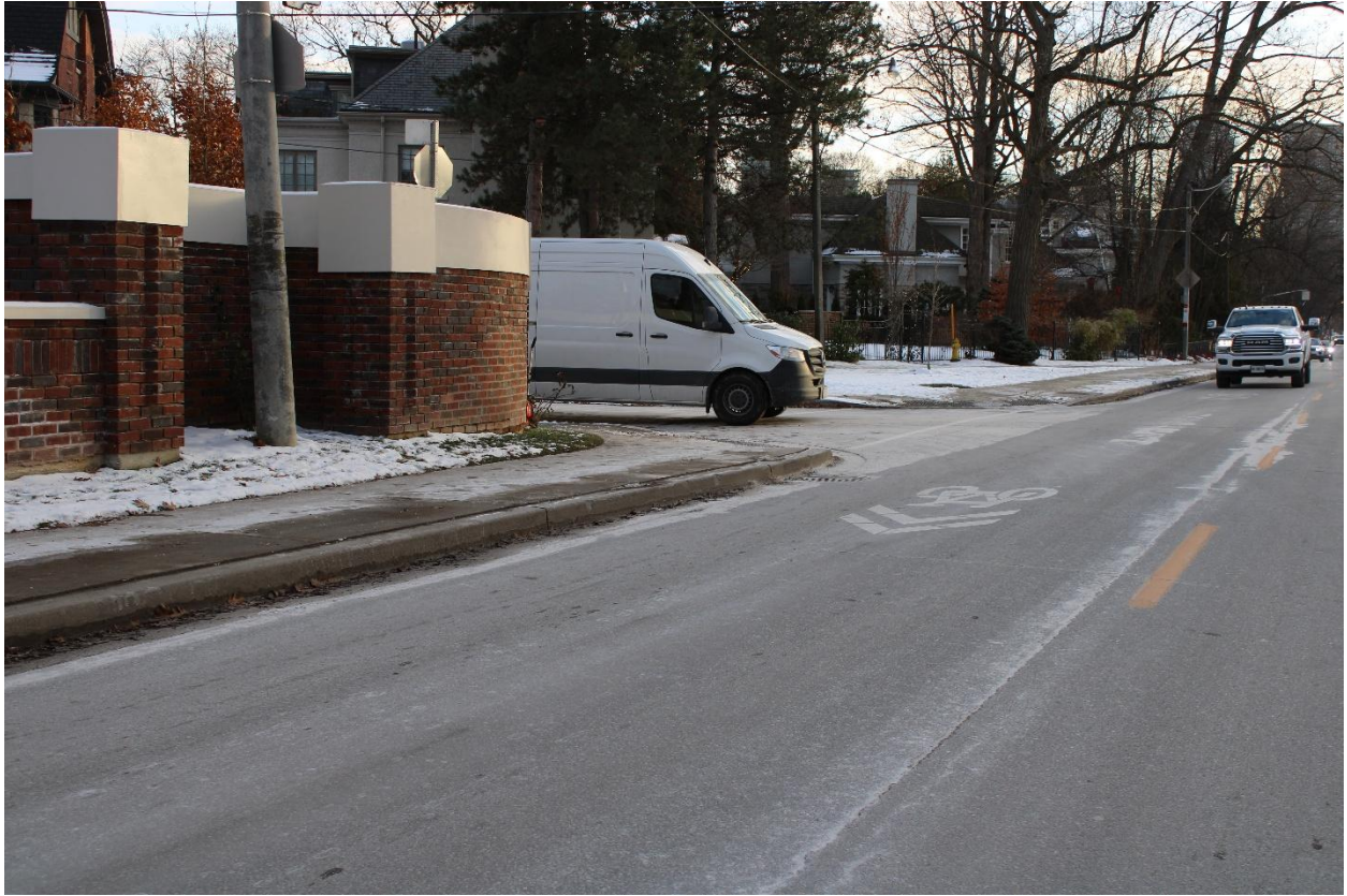
Figure 7: Site exam photo of the same large cargo van in Figure 6, taken from driver-eye height only 23 m north of the van, with the front wheels of the van now on the first pedestrian crossing line.
