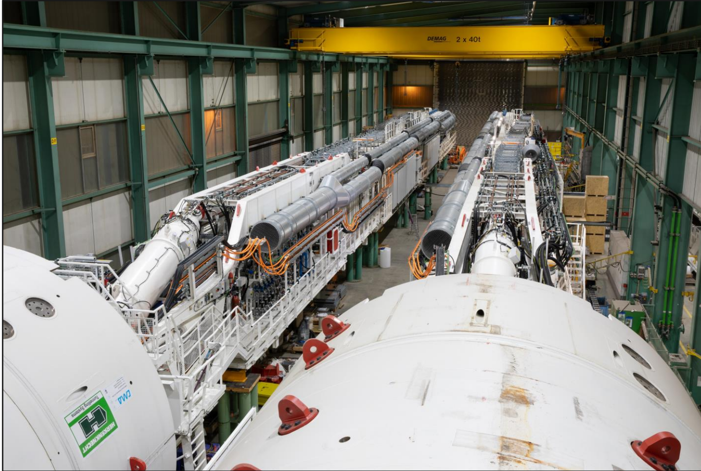
150 Meter long Tunnel boring machines factory testing
