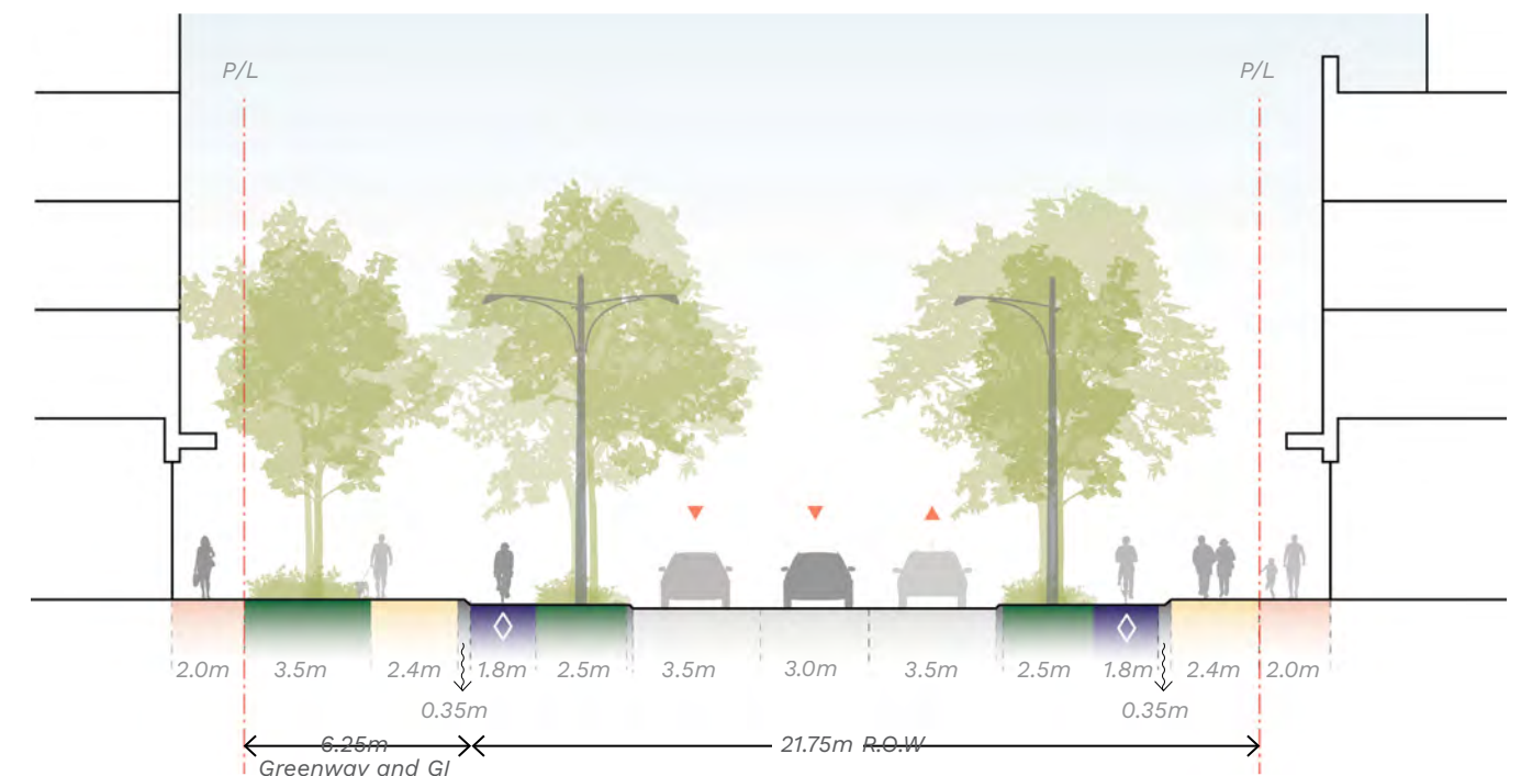
Figure 53: Typical Greenway Cross Section when adjacent to a public street.
