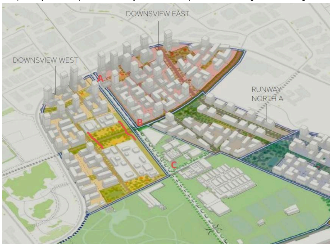
Figure 1: Demonstration Massing Plan (p107, The Framework Plan) as manually modified in red A: Downsview GO Train / Subway station (“Downsview Transit Hub”) with underground walkway B: the Northern (multi-level) Crossing created by carving out the middle section of the Supply Depot C: the Carl Hall level crossing
