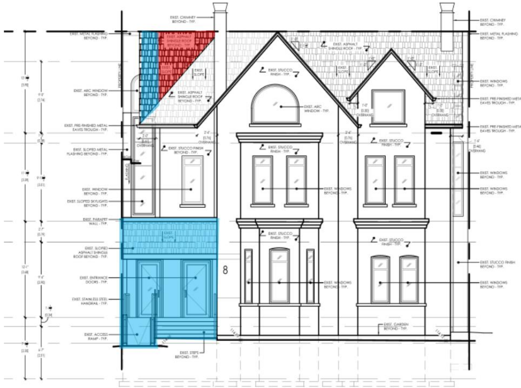
Primary (south) elevation showing alterations to the existing roof in blue and removals of the roof in red (GBCA Architects, 2026)
