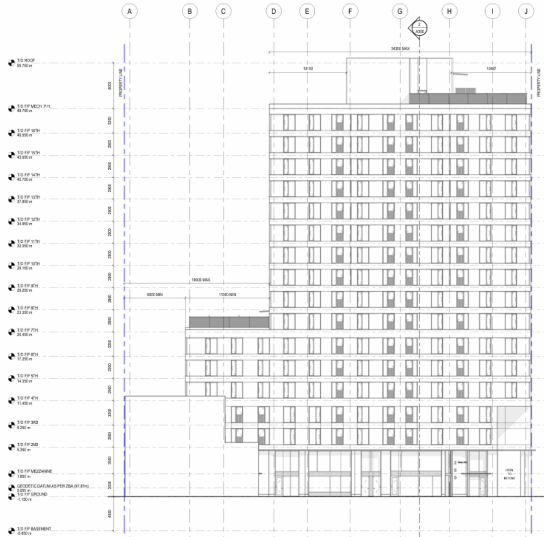
East and West elevation drawings of the new 16 storey mixed-use building with 4 storey podium building (LGA Architectural Partners Inc., 2026)
