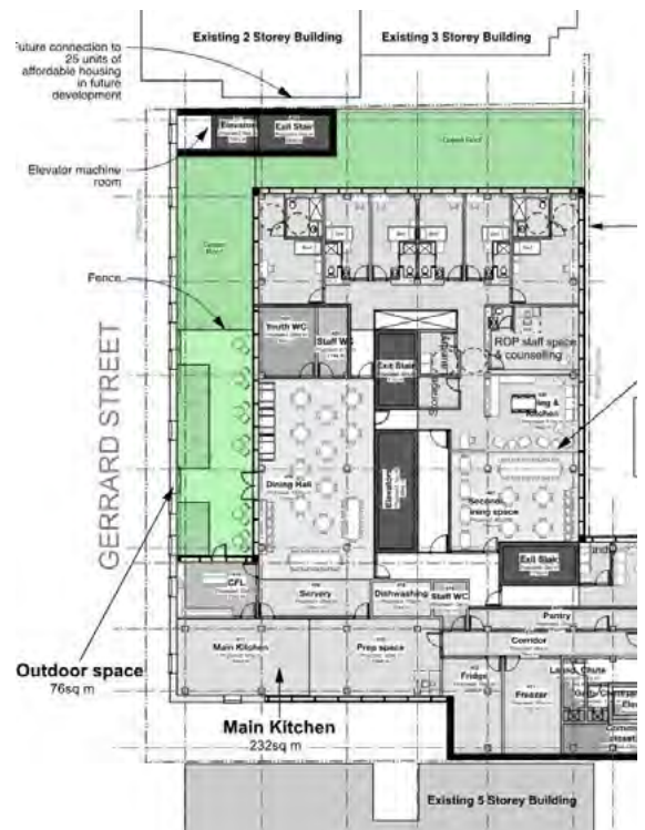
Fourth floor plan of the 20 Gerrard portion of the proposed redevelopment, showing the proposed dining terrace in green (ERA, 2026).
