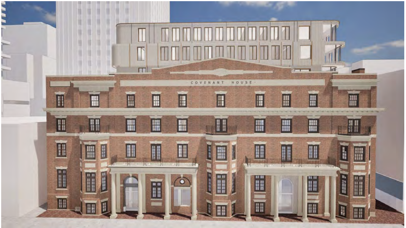
Proposed visually recessive alterations to the primary façade include the introduction of glazed guards placed in seven fourth-floor window openings, removal of WCTU lettering from the name band, and replacement of the gated opening with a curtain wall window (ERA, 2026).
