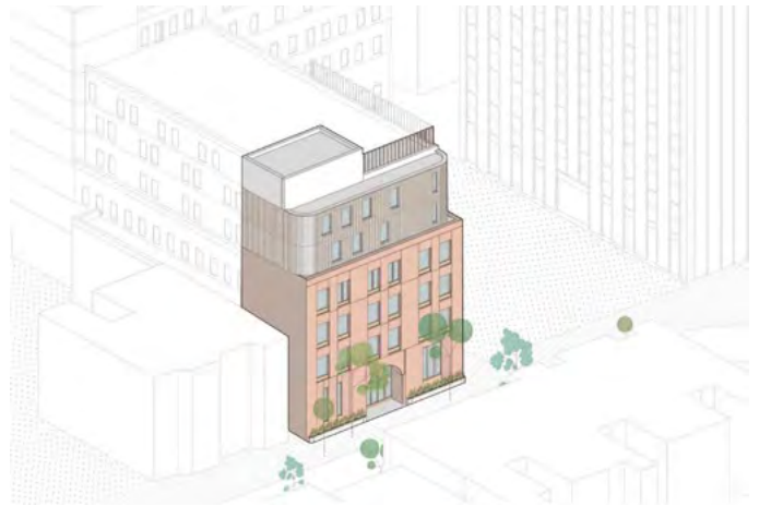
Axio view of the McGill Street portion of the proposed redevelopment, showing the proposed massing, materiality, façade rhythm, and transition from the low-rise adjacent heritage properties to the high-rise forms along Yonge Street. (ERA, 2026).
