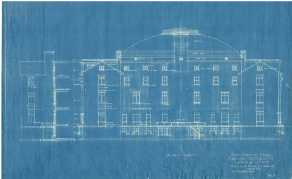
Proposed "Rear Elevation", or west elevation, of Convocation Hall, Darling and Pearson, 1904 (Source: University of Toronto Archives).
