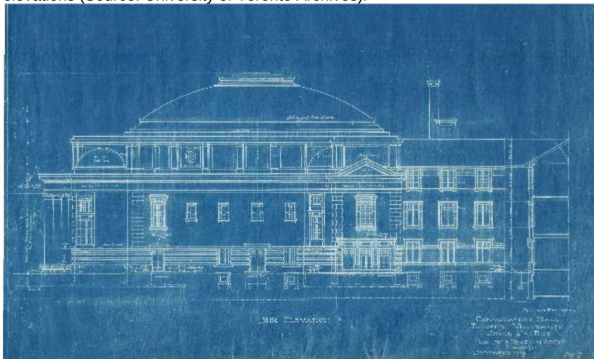
Proposed “Side Elevation”, or north elevation, of Convocation Hall, Darling and Pearson, 1904 (Source: University of Toronto Archives).
