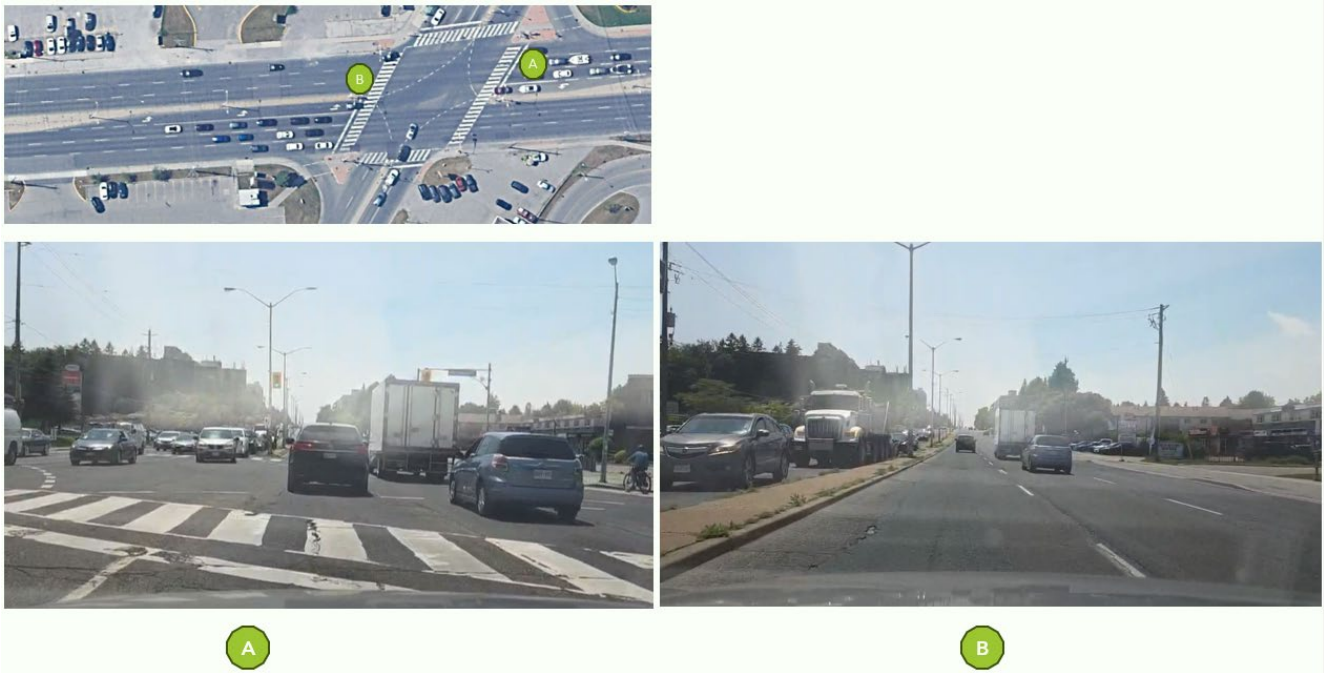
Figure 7: Site photographs illustrating westbound approach conditions, and the limited visibility of the approved JOLT display due to its location, viewing angle, and obstruction by opposing traffic.
