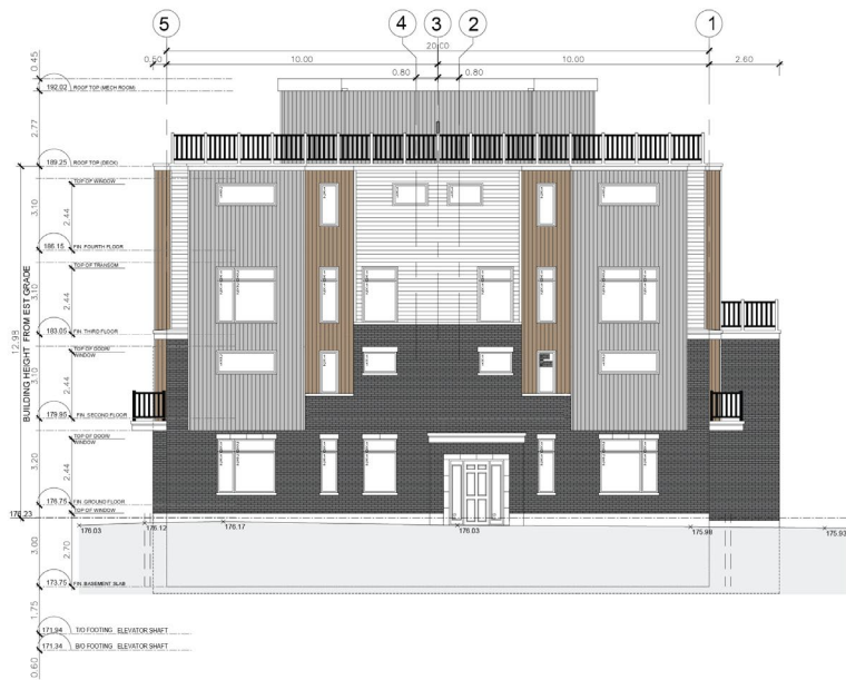
Buildings A - West Elevation
