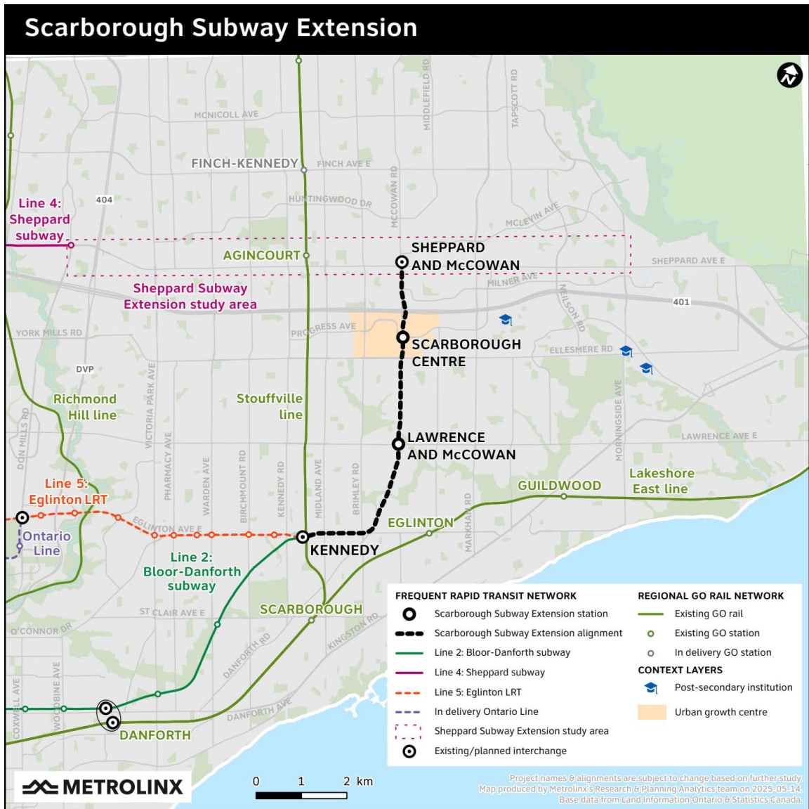
Figure 1: Scarborough Subway Extension Alignment (Source: Metrolinx)
