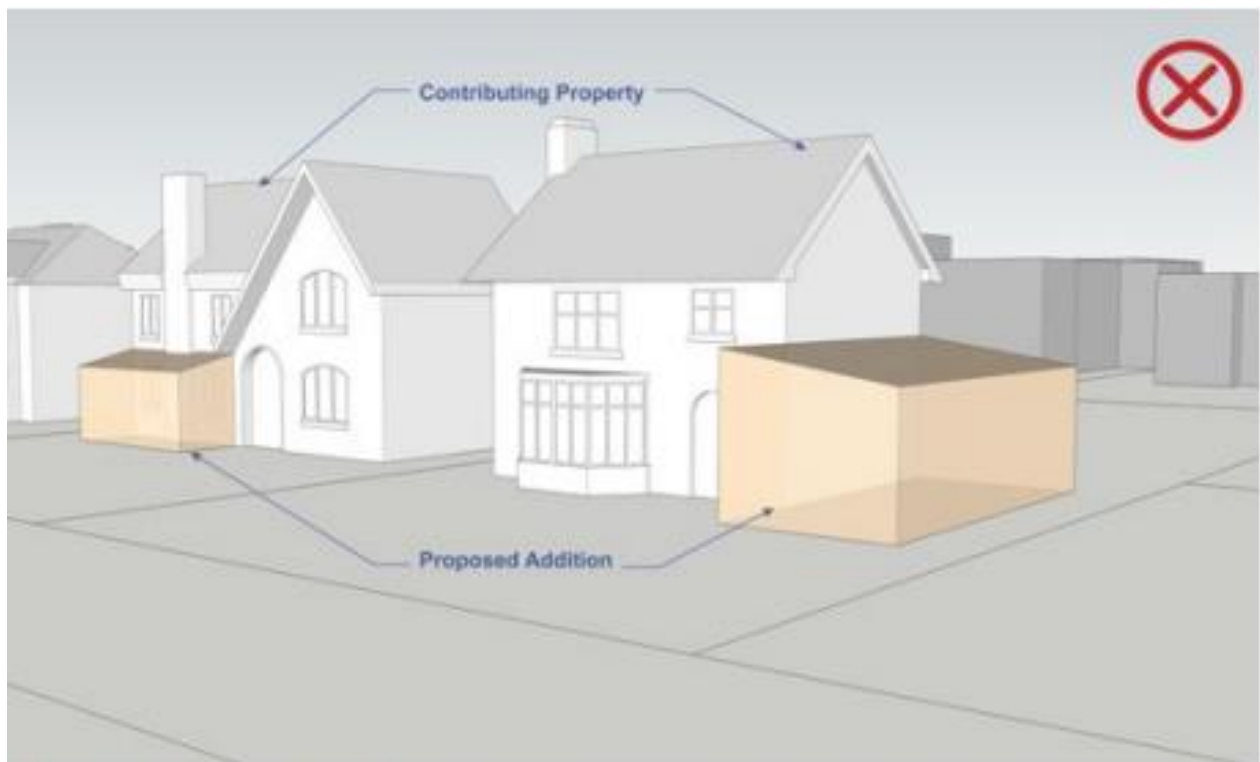
Figure 37: Contributing Property - incompatible addition (view from street).
