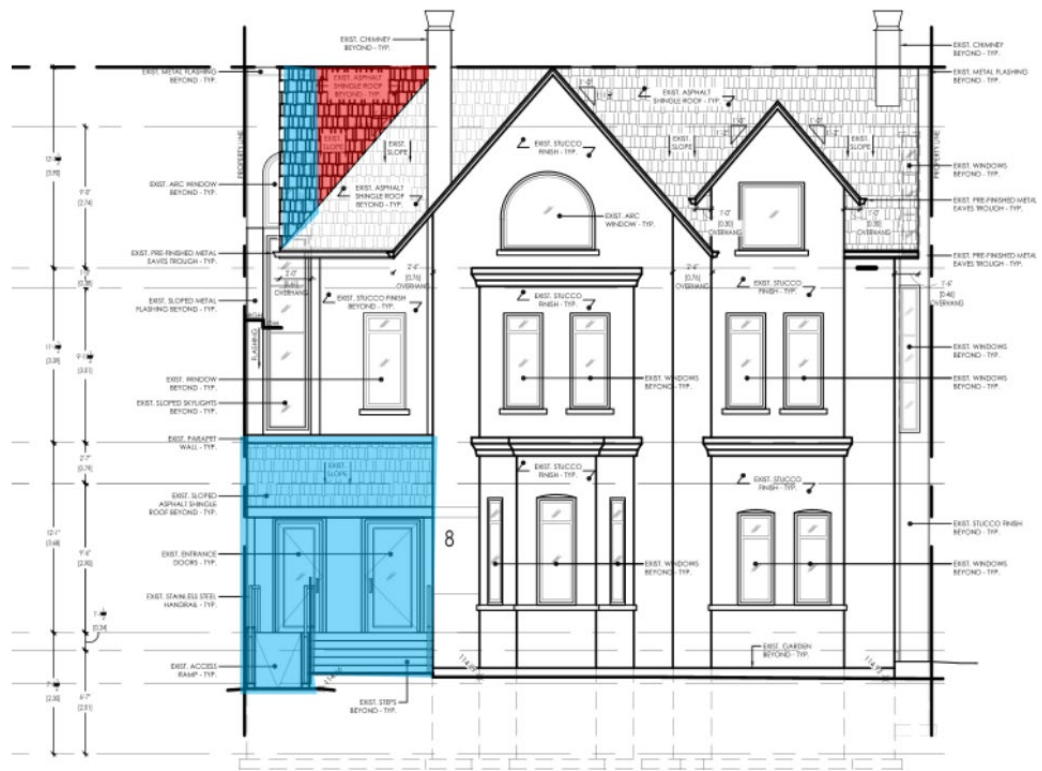
Primary (south) elevation showing proposed alterations to a portion of the sloped roof to be demolished in red and the alterations proposed to the roof of the main entrance on the side shown in blue (Source: GBCA Architects, 2026)
