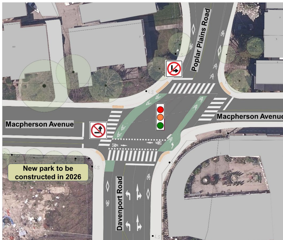
Figure 3: Proposed intersection safety improvements at Davenport Road and Macpherson Avenue and Poplar Plains Road
