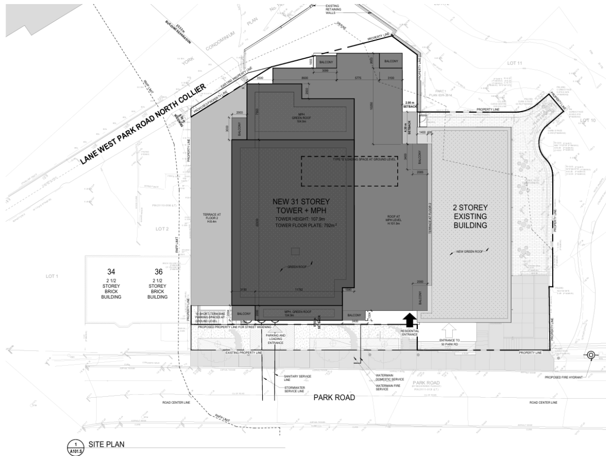
Site Plan drawing showing heritage building at 50 Park Road in red outline and proposed 31 storey new tower building at 38-40 Park Road (BDP Quadrangle, 2025).
