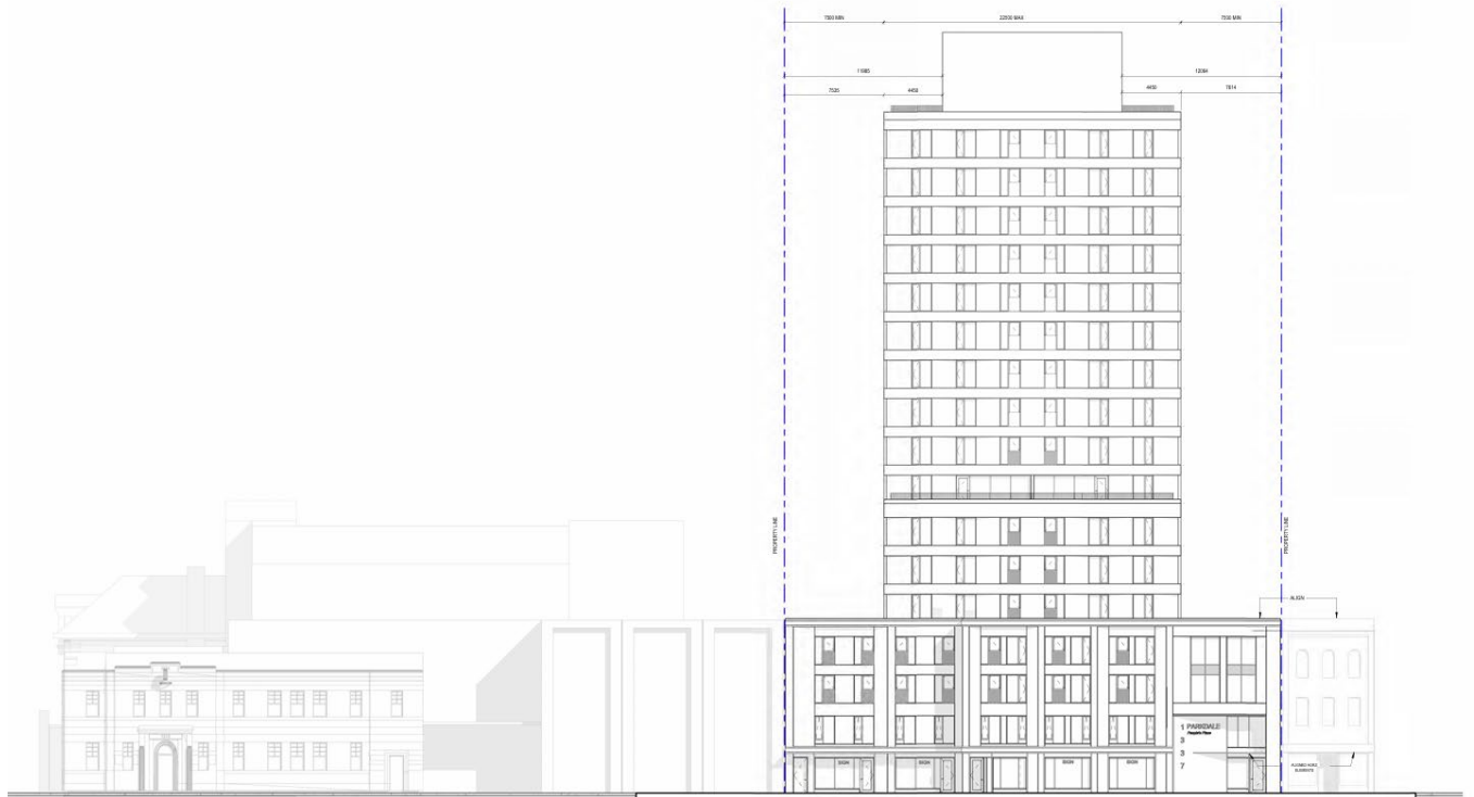
North elevation drawing of the Parkdale Hub project showing the proposal of the West Block and reference to the Centre Block proposal (LGA Architectural Partners Inc., 2026)
