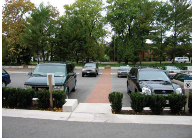
Pedestrian connections should connect buildings to the public realm and should create safe paths of travel for pedestrians through parking areas.
