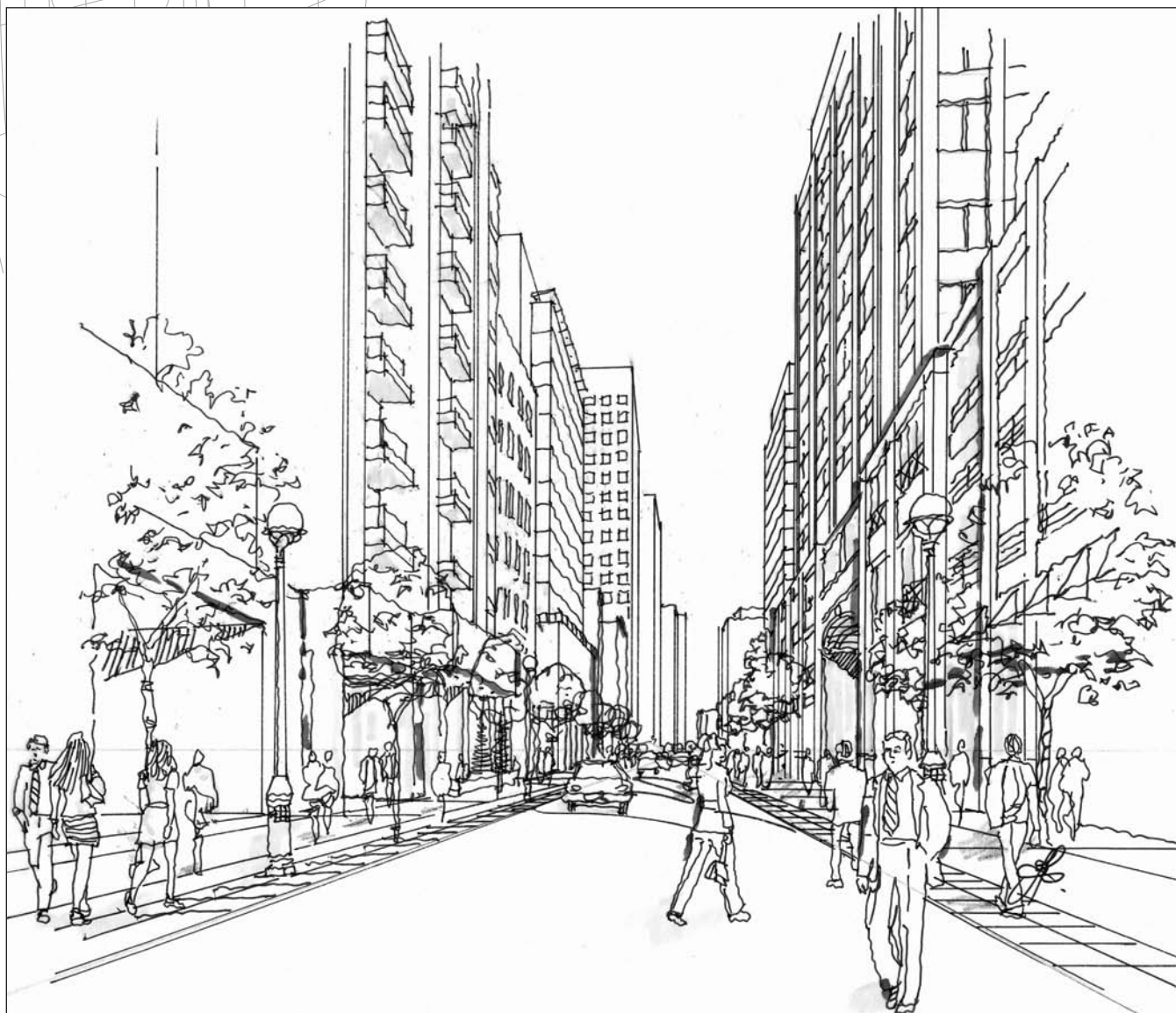
Figure 7: Hayden Street sketch looking east along Hayden Street showing buildings with mid-block connections, consistent setbacks, and step backs above a podium
