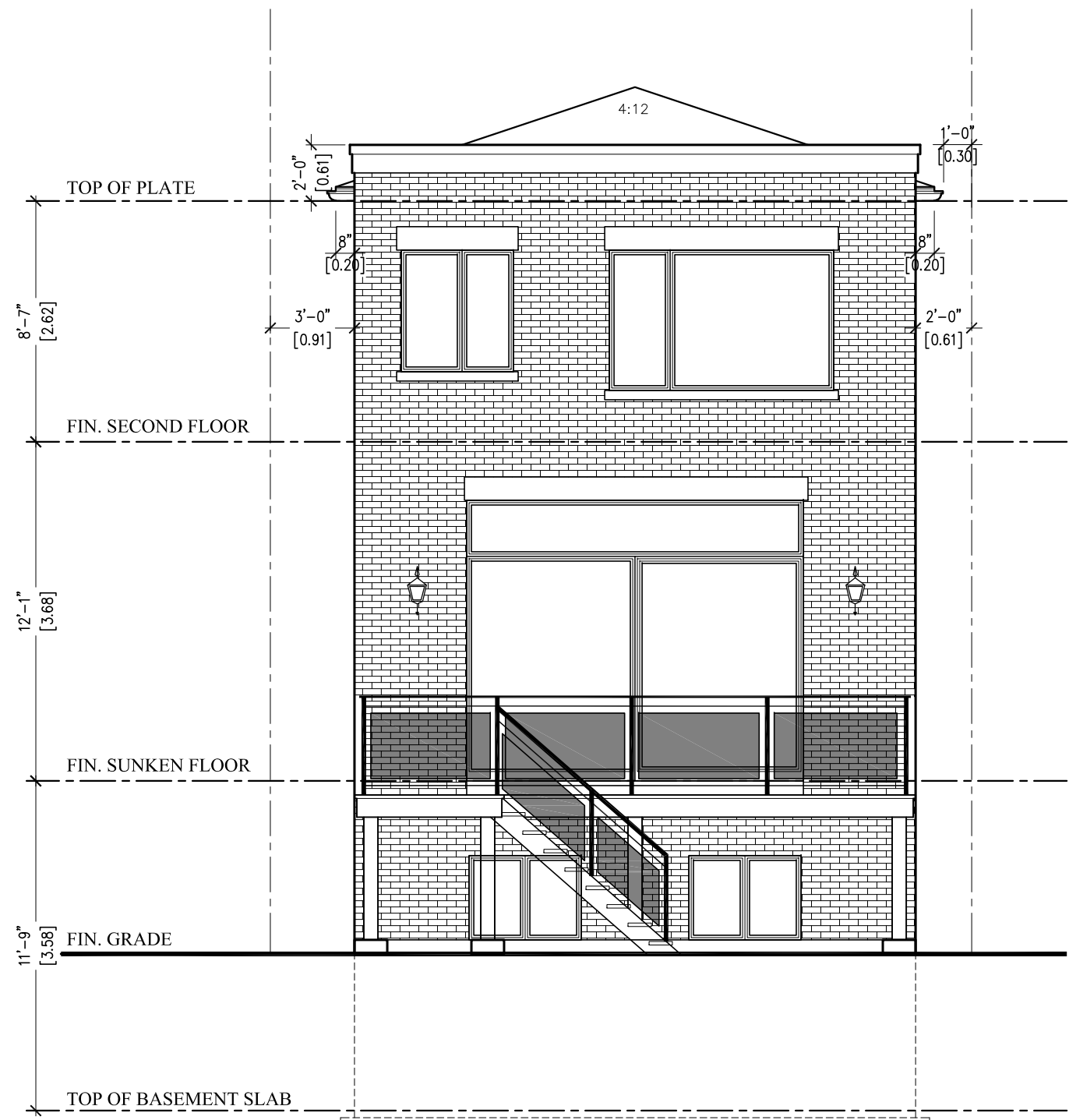
REAR ELEVATION PART1 (SOUTH) 3/16"=1'-0"
